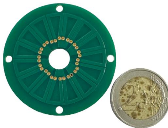
Fig. 3.17 Axial flux PCB stator comprising six layers
