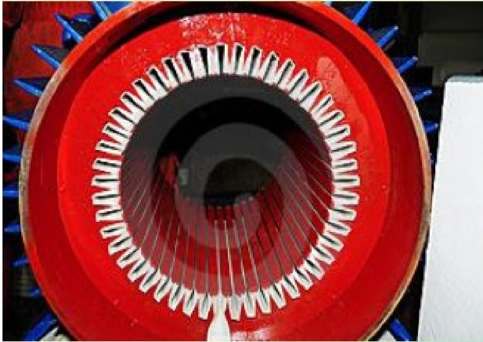
Figure 3.1 Stator of a three-phase induction motor.
