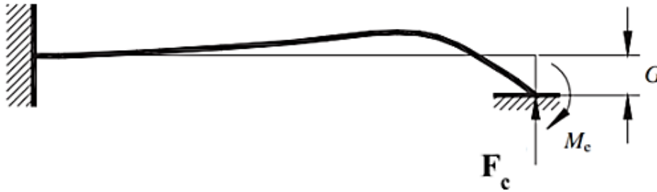
Figure 13. Contact force acting at switch contact region [41]
