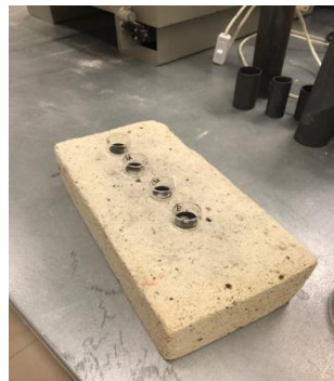
Figure 2.2: Air-annealing on four test samples in the quartz cups at same temperature.
