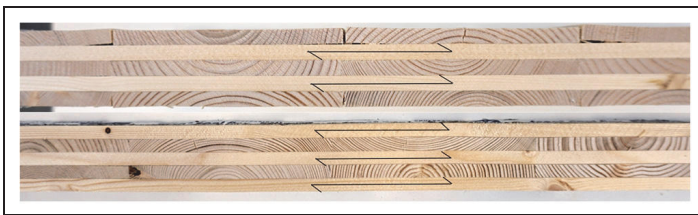
Figure 7. Cross-section of the five-layer and without edge-bonded panels (WBE5L) from the narrow side (top) and the long side (bottom), cut after the final conditioning step (RH 15%).
