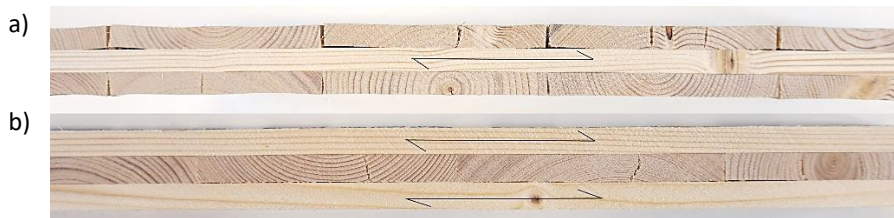
Figure 4.3. Cross-sections of 3-layer and without edge-bonded panel (WBE3L) after the final conditioning step at RH of 15 %, the narrow side (a) and the long side (b) of the panel.
