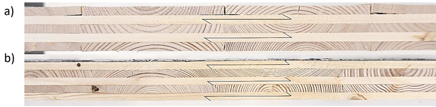
Figure 4.4. Cross-sections of a 5-layer and without edge-bonded panel (WBE5L) after the final conditioning step at RH of 15 %, the narrow side (a) and the long side (b) of the panel.
