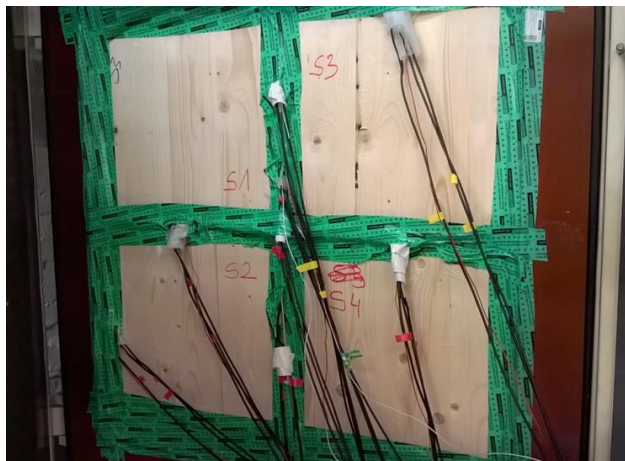
Figure 3.1. CLT specimens placed inside the climate chamber ILKA PTK-3018 doorway.
