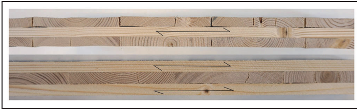
Figure 6. Cross-sections of the three-layer and without edge-bonded panel (WBE3L) from the narrow side (top) and the long side (bottom), cut after the final conditioning step (RH 15%).
