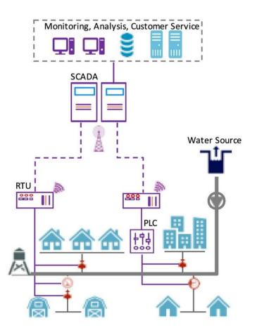
Figure 1:Typical architecture of a water-supply system (Source [6])
