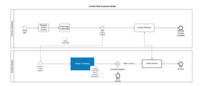
Figure 15: Blockchain risk security control on the SCADA system
