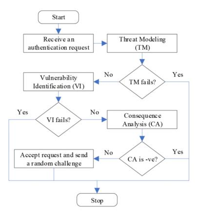
Figure 6: Security measure flowchart for CyRA (Source: [29]).
