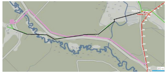
Fig. 5. 15 kV solution for Holdre substation feeder 1.
