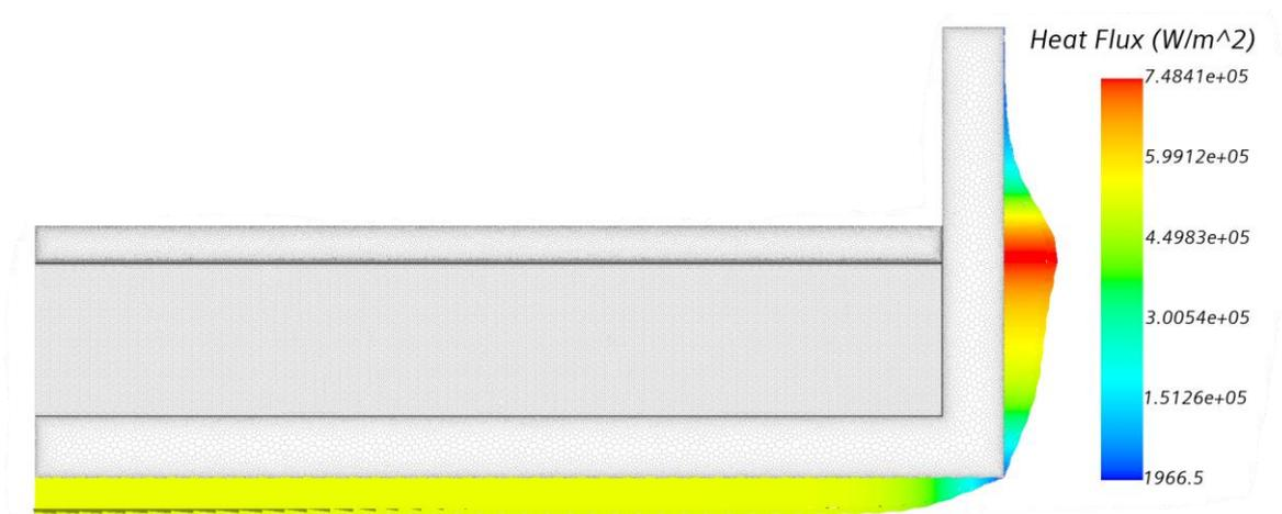
Figure 2.14: Outer heat flux profile of the RPV
