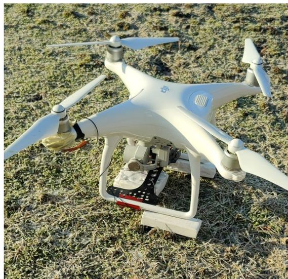
Figure 1. *An image of the Drone with the payload system attached*
