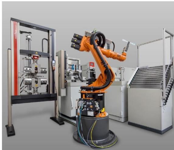
Figure 19. RoboTest R robotic testing system (Polar) for metals [17].
