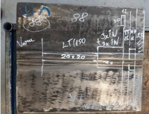
Figure 12. Manually marked cuttable Butt Joint Weld specimen positions
