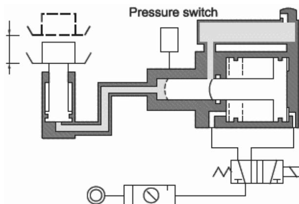
Figure 18. Hydro Pneumatic Booster Cylinder [14]
