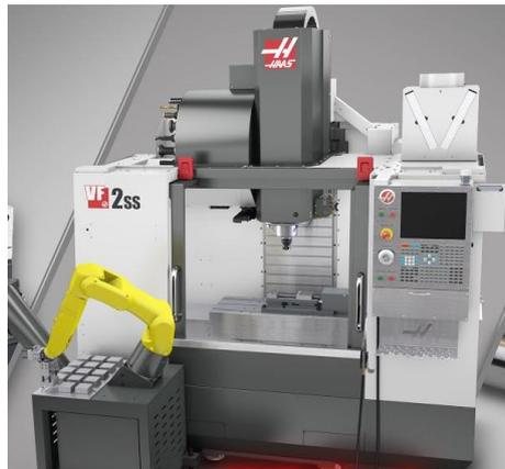
Figure 6. Haas HRP-1 Robot package [6]
