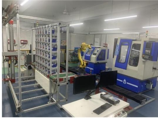
Figure 9. One robot serves multiple stations [8]
