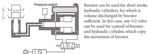
Booster can be used for short stroke hydraulic cylinders, for which is volume discharged by booster sufficient. In this case, any 5/2 valve can be used for control of booster and hydraulic cylinder, which copy the movement of booster.
