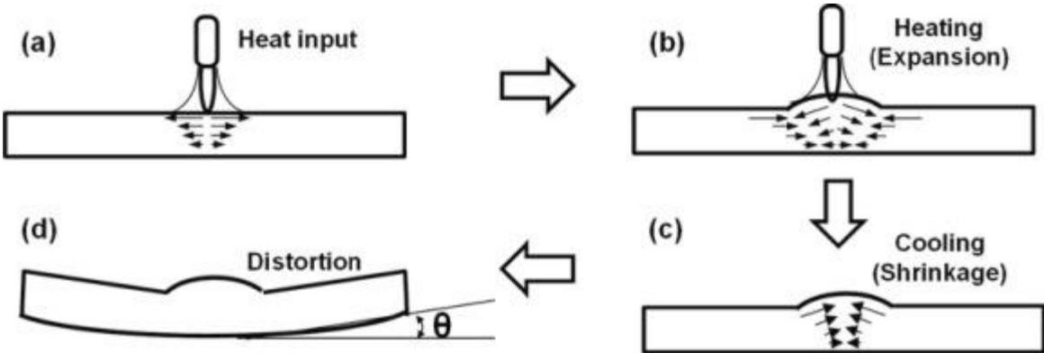
Figure 1. Welding Deformation in Butt welding [4].
