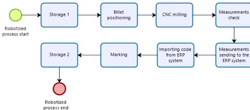
Figure 4. Automated general process sequence
