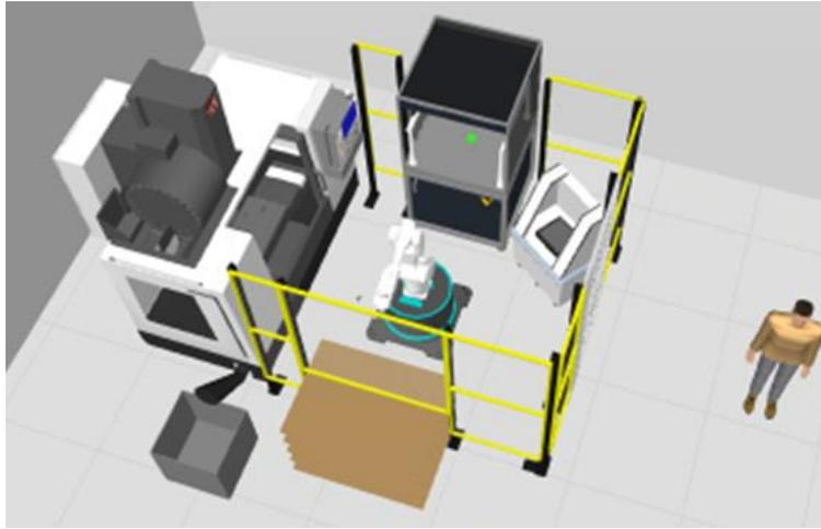
Figure 3. Concept 1 robot cell with separate system parts
