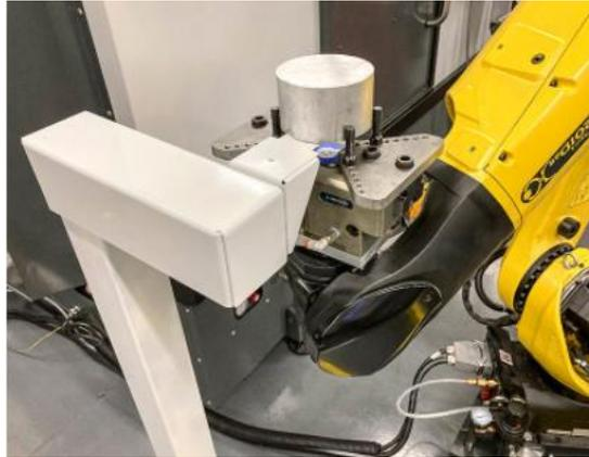
Figure 21. Part Flipping Station [19]
