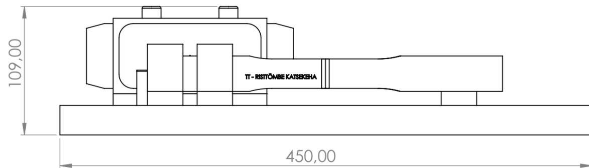
Hydraulic piston presses the specimen against the support 2
