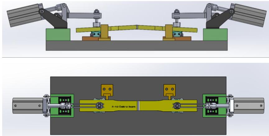
Figure 16. Custom Jig 1 conceptual idea (Graphical material 2)
