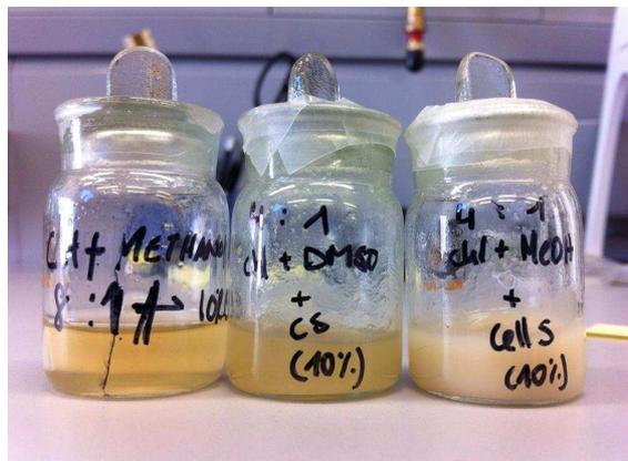
**Figure 38. Examples of electrospinning mixtures. The one on the left is suitable for electrospinning, the one in the middle is too viscous and the one on the right, the polymer is precipitated.**
