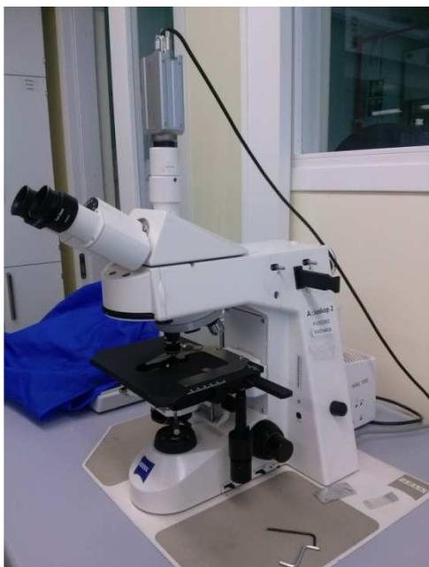
Microscope used for evaluation of electrospinning results.
