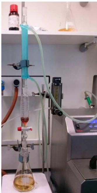
**Figure 10. Setup for Cellulose Stearate obtention.**
