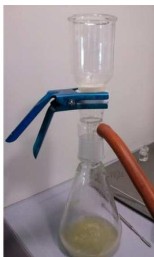
**Figure 12. Filtration under vacuum setup.**
