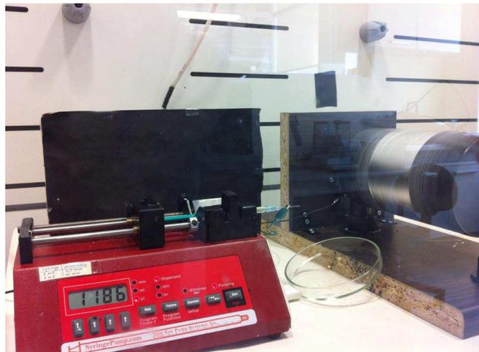
**Figure 39. Electrospinning setup.**
