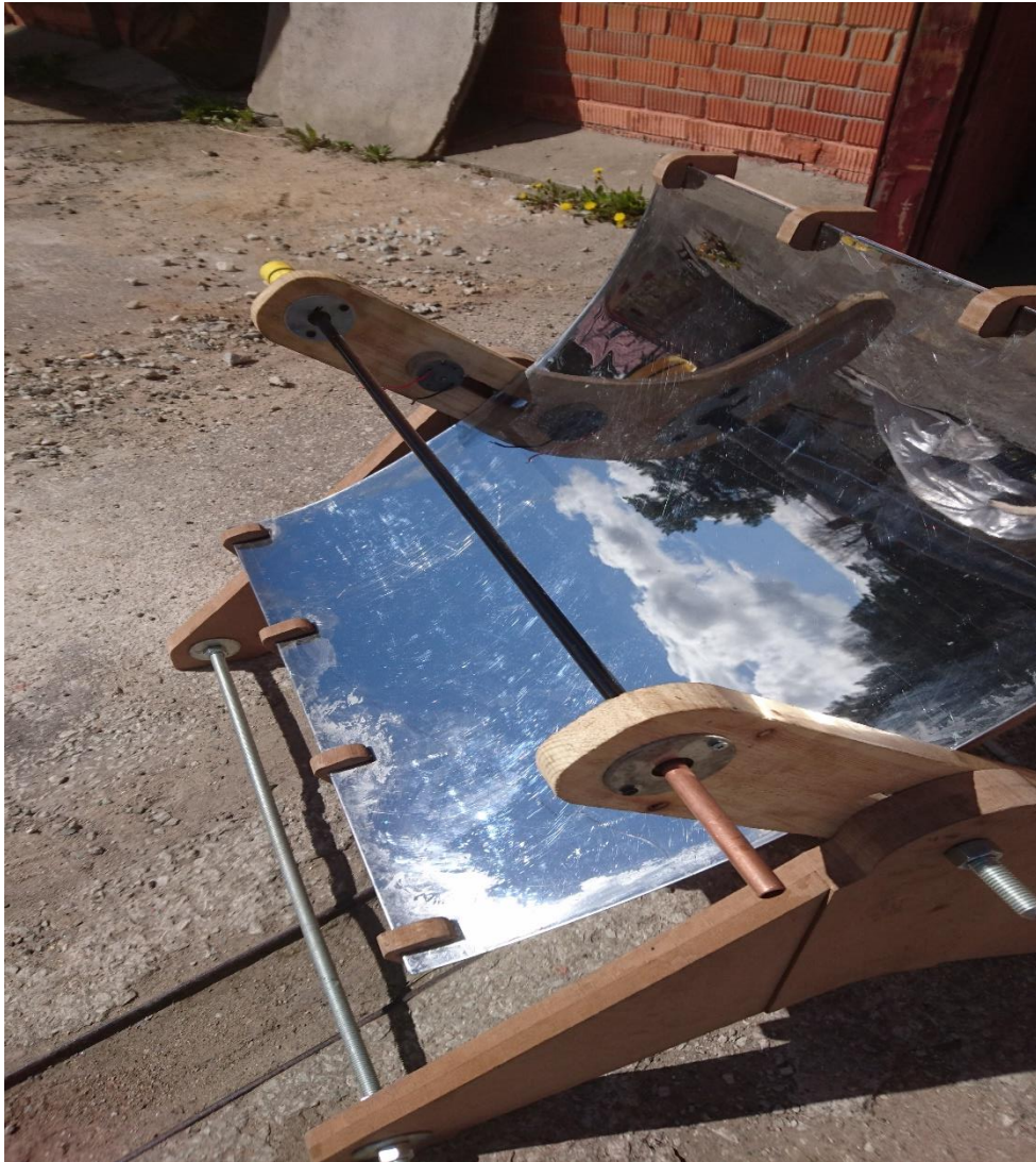
Figure 34. Receiver of designed trough without glass coating for isolation. Taken by author
