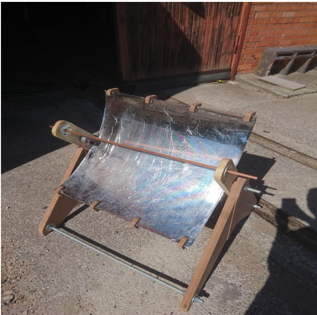
Figure 27. Trough with protective layer. Taken by author.
