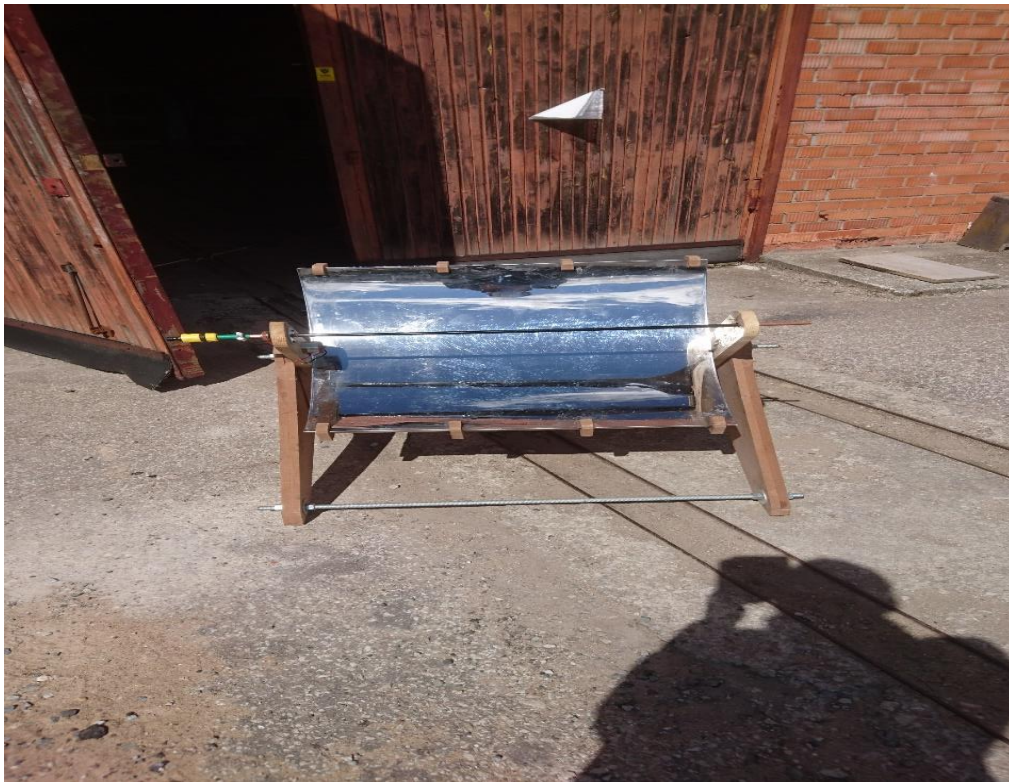
Figure 28. Trough without protective layer. Taken by author
