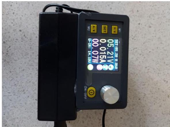
Figure 32. DC-DC Converter.
