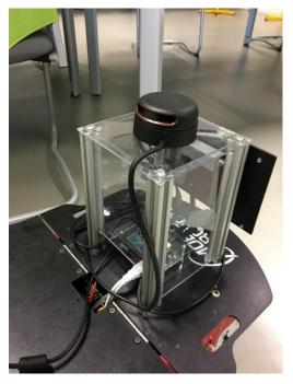
Figure 3.5 RPLIDAR mounted on the Pioneer 3-DX robot
