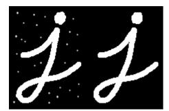
Figure 5.7 The result of performing cv2.erode() and cv2.dilate() functions. On the left side is an image before performing functions. (7)
