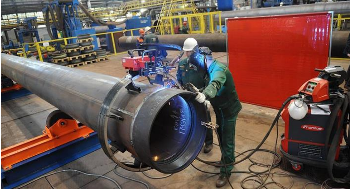
Figure 7. An example of orbital welding [3].
