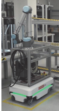
Fig. 4. Robot arm and mobile robot tandem.
