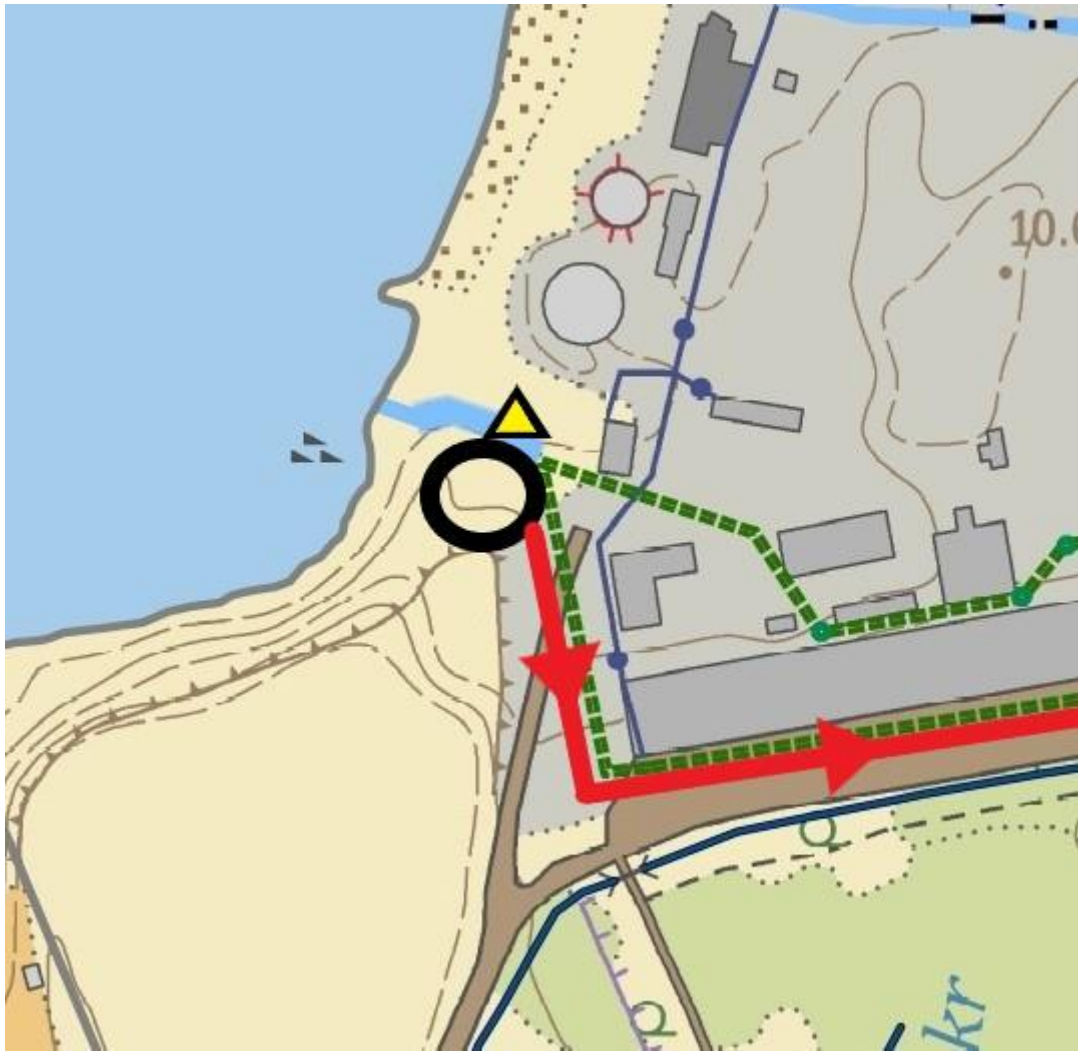
Figure 3.14. Proposal for the Area 3. The black circle represents the storage tank and the belt oil skimmer, the yellow triangle will be the location of the flow-meter and the continuous probe, and the red line is the pipe that connects the water storage tank with the beginning of the Area 2.
