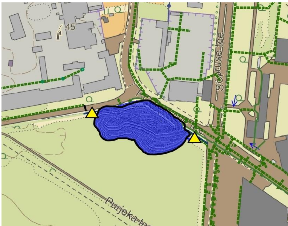
Figure 3.9 Technical solution consisting of a Surface Constructed Wetland (in blue). The yellow triangles represent the flow-meters and the continuous probes located both at the inlet and the outlet.
