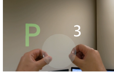
(b) Interaction with the PI tuning spheres: Next, the sphere is resized by bringing the hands closer together or moving them further apart from each other.
