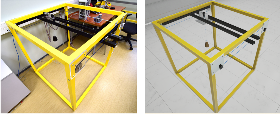
(a) Real-life 3D crane control object, courtesy of the Center for Intelligent Systems at Talltech. (b) 3D Model of the 3D crane control object.
