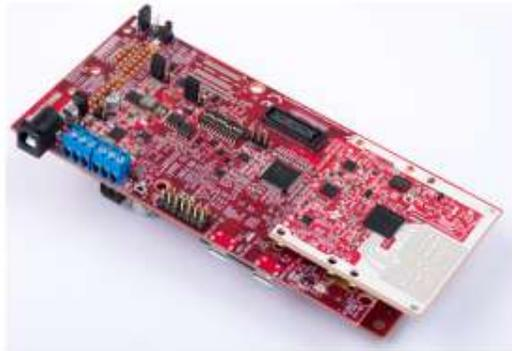
Figure 38. IWR6843ISK mmWave sensor on its carrier platform MMWAVEICBOOST
