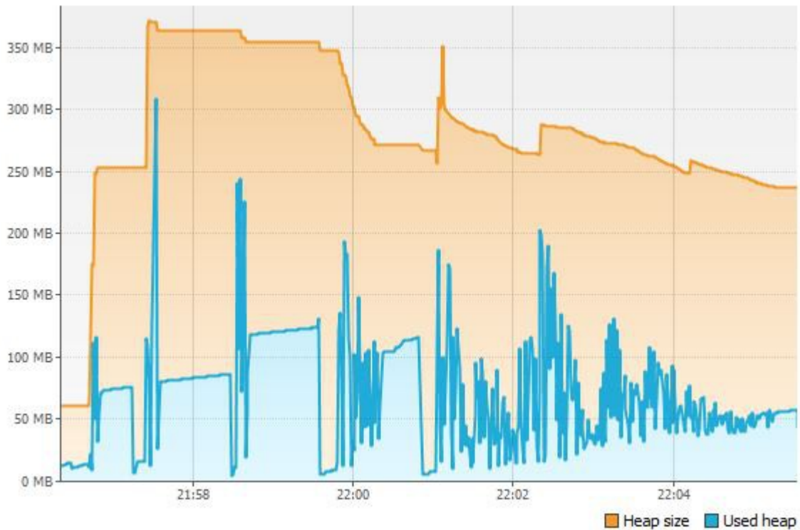
Illustration 9: MONSABAN memory usage while processing Mushroom 19-column dataset (complete run: MONSABAN, DSR, Unique + greedy coverage algorithm). Illustration is made using Virtual VM software.
