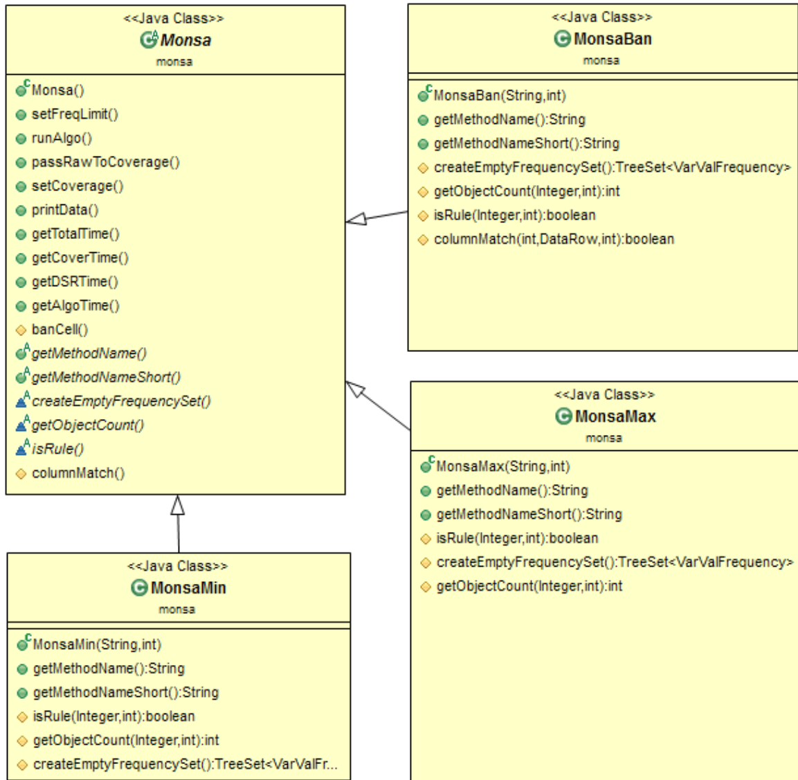
Illustration 10: Class diagram demonstrating the differences in implementation for MONSA algorithms. Private methods are omitted.
