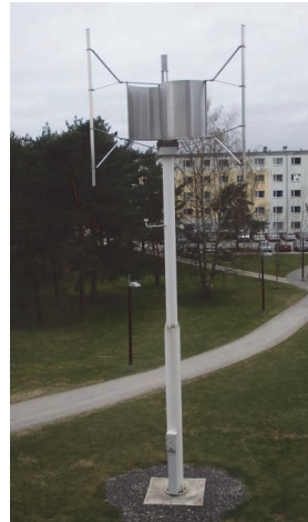
Fig. 13. Prototype generator installed into vertical axis wind turbine.
