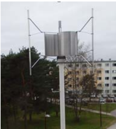
Fig. 2.2. The combined wind turbine, which consist of Darrieus and Savonius turbines.
