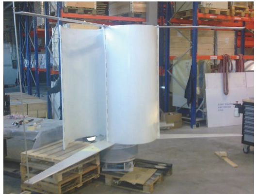
Fig. 16. Generator with half-assembled H-type wind turbine (with savonius).
