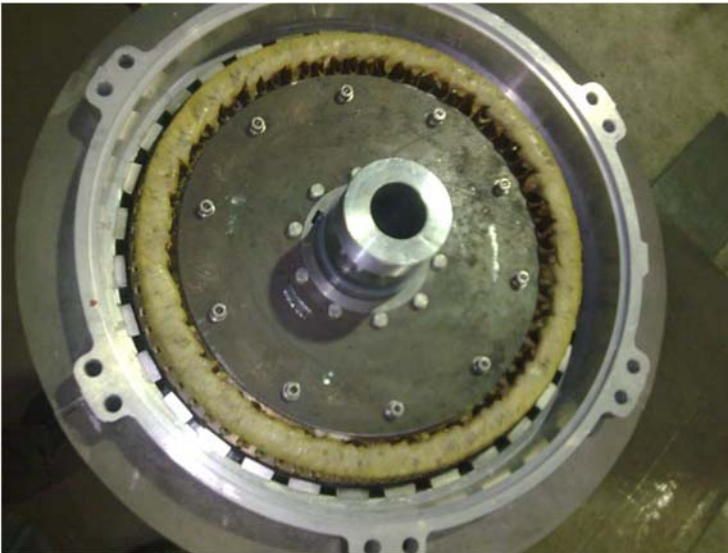
Fig. 8.5. A photo of the 5 kW permanent magnet generator with outer rotor.
