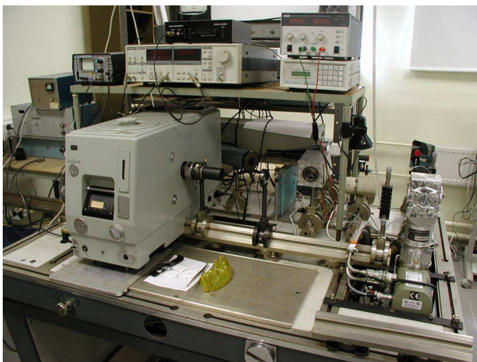
Figure 3. Experimental setup of photoluminescence measurements at Tallinn University of Technology.
