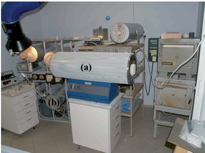
Figure 9. Photo of the used furnaces, a) for the isothermal arrangement, b) for the two-zone arrangement.
