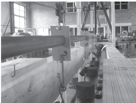
*Figure A.1.13. Deformed stiffening girder in the unloaded span*
