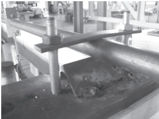
*Figure A.1.2. Support of the stiffening girder (in the middle)*
