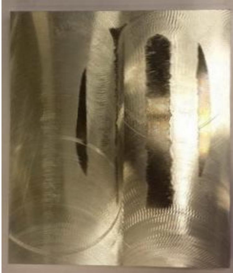
**Figure 23 - Curved channel 1 after surface milling.**
