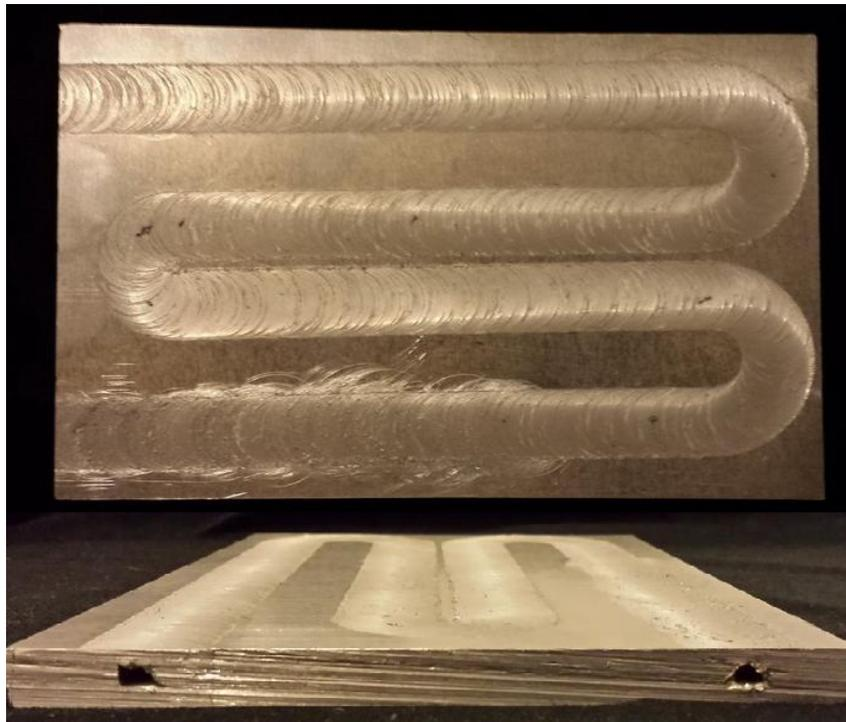
Figure 24 - Curved channel 2 produced by position control.
