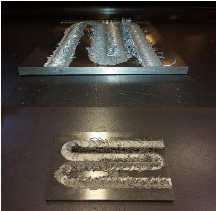
Figure 22 - Curved channel 1 produced by force control.
