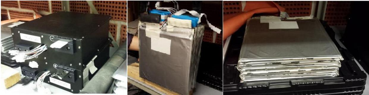
Figure 27 Industrial lithium battery and battery cells.
