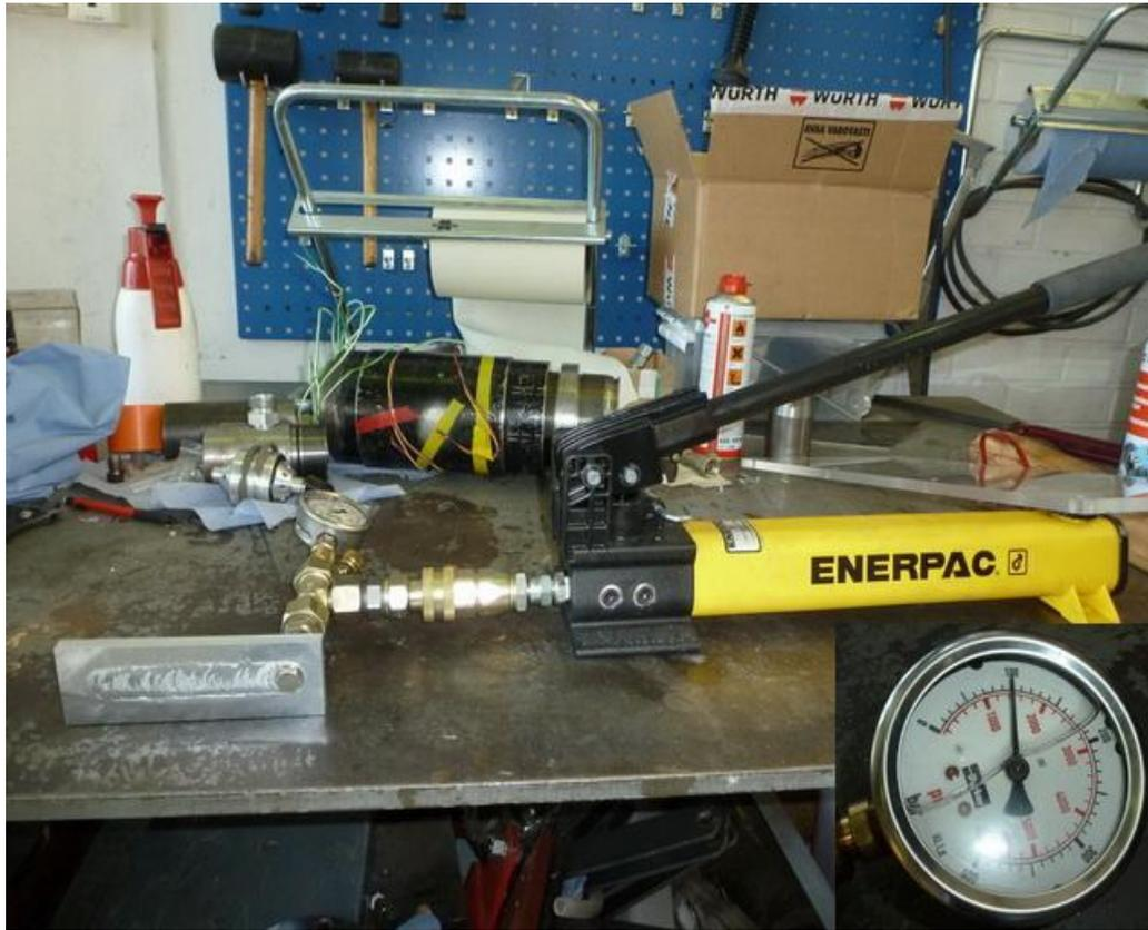
Figure 41 - Equipment for hydraulic test.
