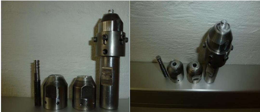
Figure 15 - Shoulders, Probe and assembly of the tool
