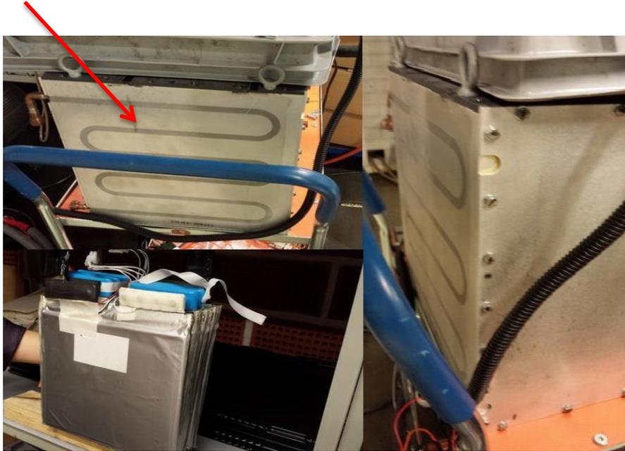
Figure 30 - Cooling system of industrial lithium battery.
