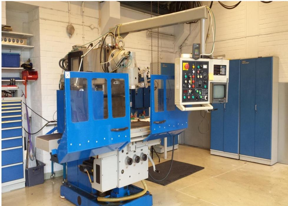
Figure 16 - CNC milling machine used for producing straight FS channel.
