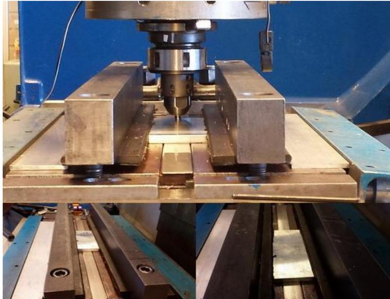
**Figure 18 - Clamping of workpiece on machine table.**
