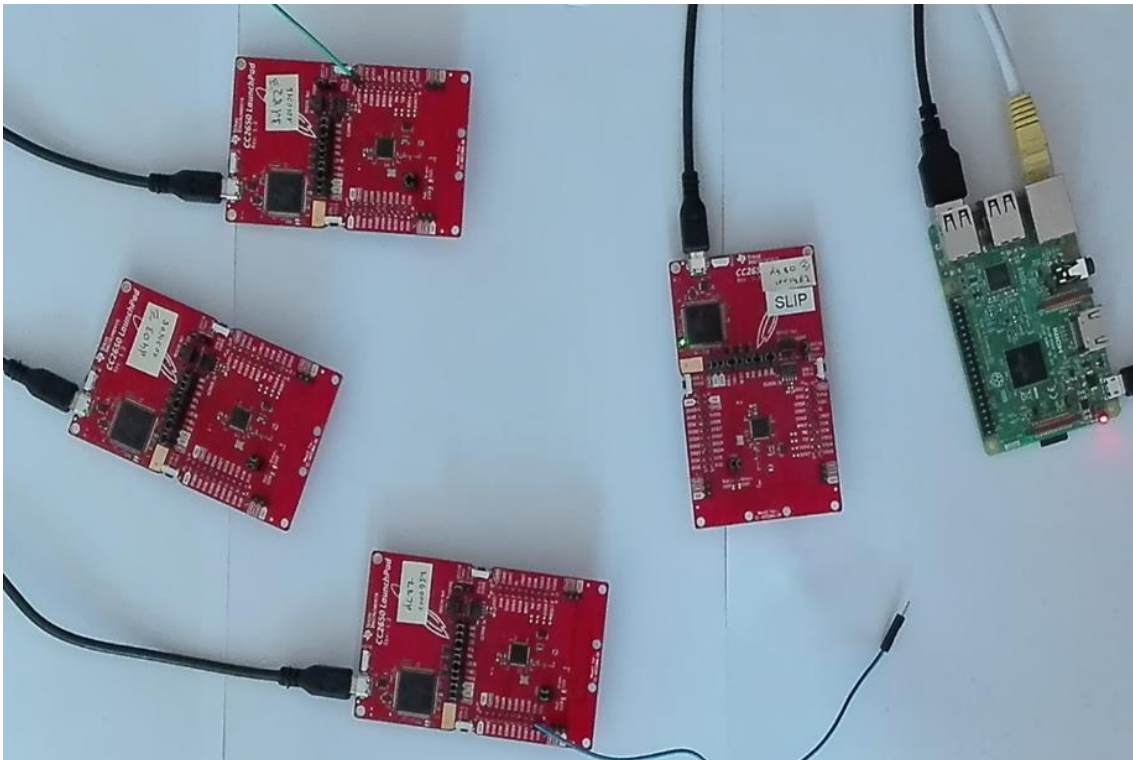
Figure 10. Complete 6LoWPAN test setup.
