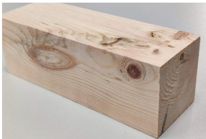
Figure 2.7 An example of a C-grade block, cross-section 58x58mm
