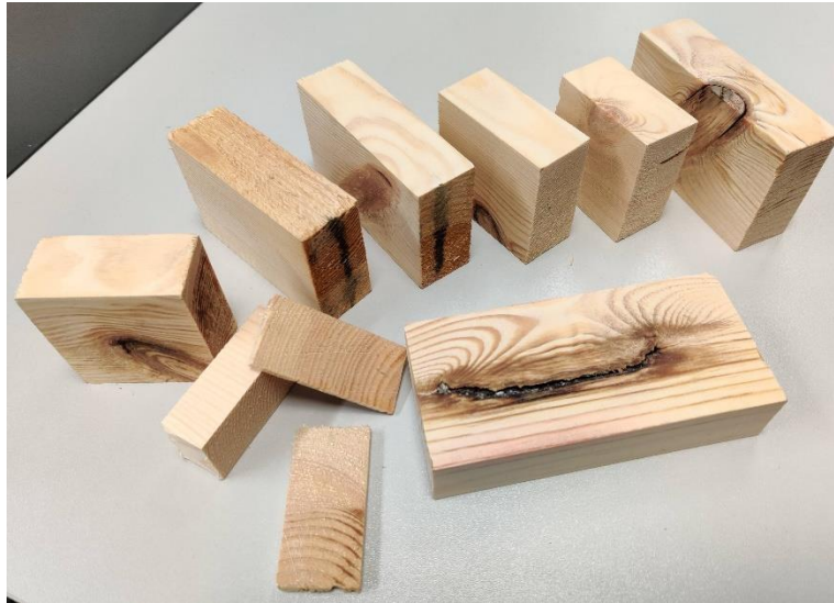
Figure 2.8 An example of reject pieces – end-cuts, undersize, large defects
