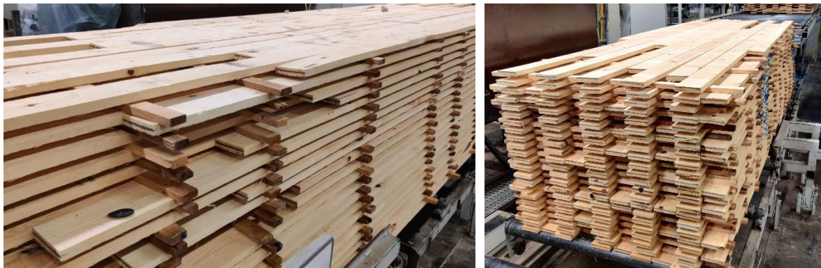
Figure 4.1 Typical board-type sawn timber, cross-section 25x125mm
