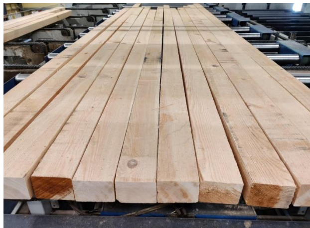
Figure 4.2 Typical stud-type sawn timber, cross-section 56x73mm
