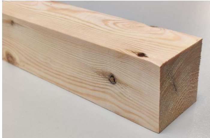
Figure 2.5 An example of a B-grade block, cross-section 58x58mm
