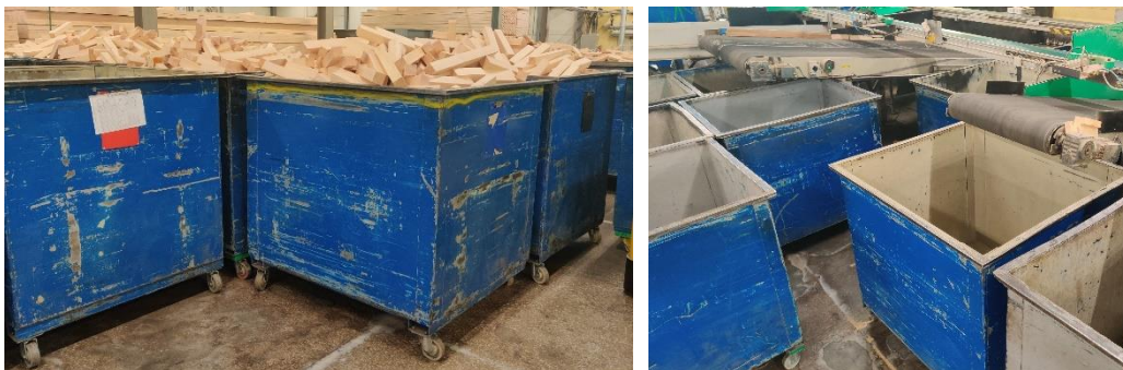
Figure 2.9 Metal containers as buffer room between cross-cutting and finger jointing
