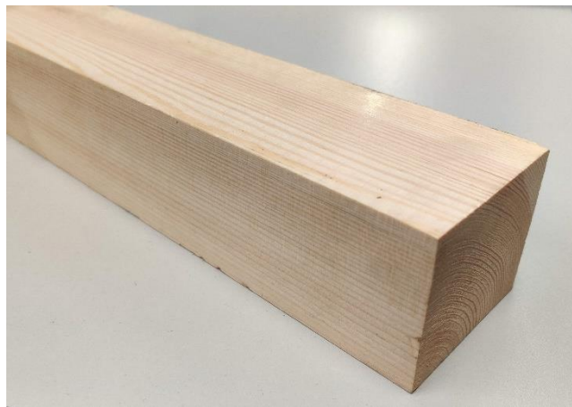
Figure 2.3 An example of an A-grade block, cross-section 61x72mm
