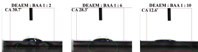
Figure 3.3 Droplets of ultrapure water on the polymer surfaces prepared with the different DEAEM/BAA ratios.
