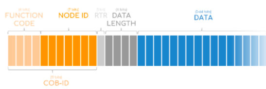
Figure 2.1.2. CANopen frame work [19]
