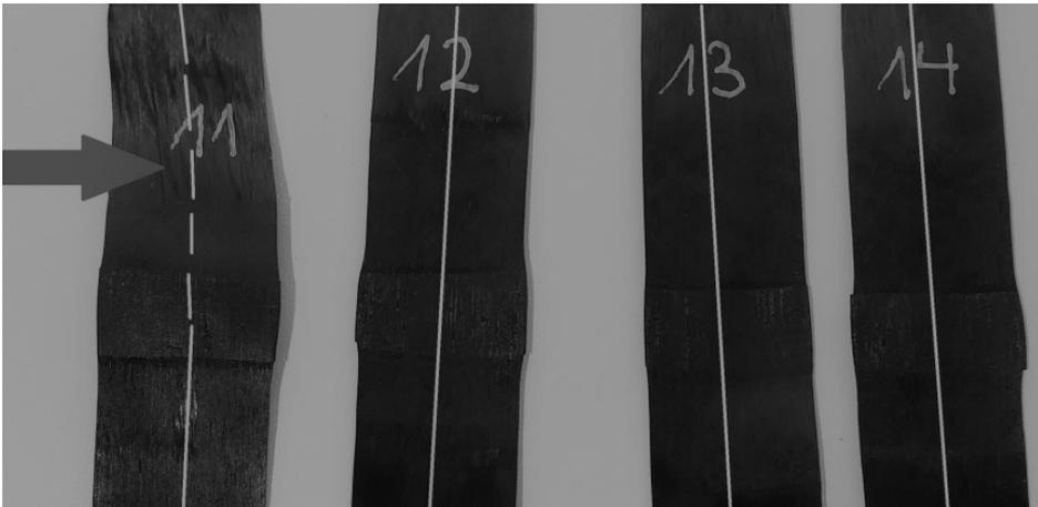
*Figure 3.7 Deformed specimen no.11.*
