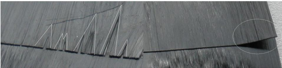
**Figure 3.4.** Defects in the laminate. Evaporation of the matrix material on the left and improper adhesion on the right.
