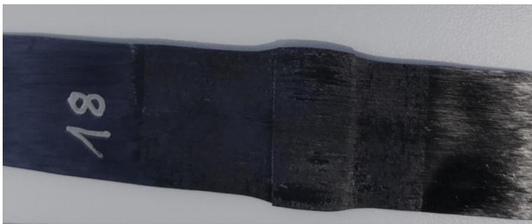
**Figure 3.9** *Result of an excessive compaction force.*
