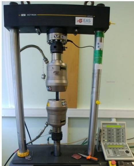
**Figure 2.12** Specimen in the tensile- compression machine.
