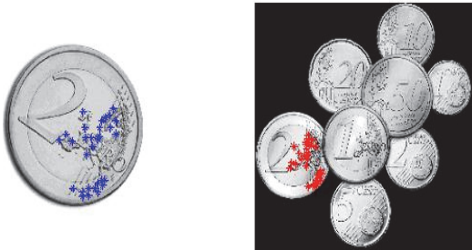
Figure 3. Rotated 2 Euro coin detection with SIFT feature method.
