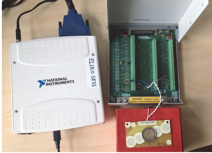
Figure 2.4. Working setup for conductivity evaluation.
