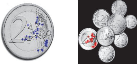
Figure 2. 2 Euro coin detection with SIFT feature method.
