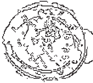
Figure 4.19. Frame after canny edge detector [II (81)].
