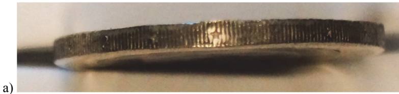
Figure 4.13a) Image of coin edge, b) processed image of the edge of counterfeit coin (Germany).
