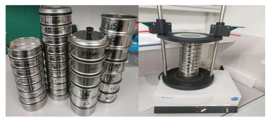
Figure 2.1 Scheme of sieving machine.
