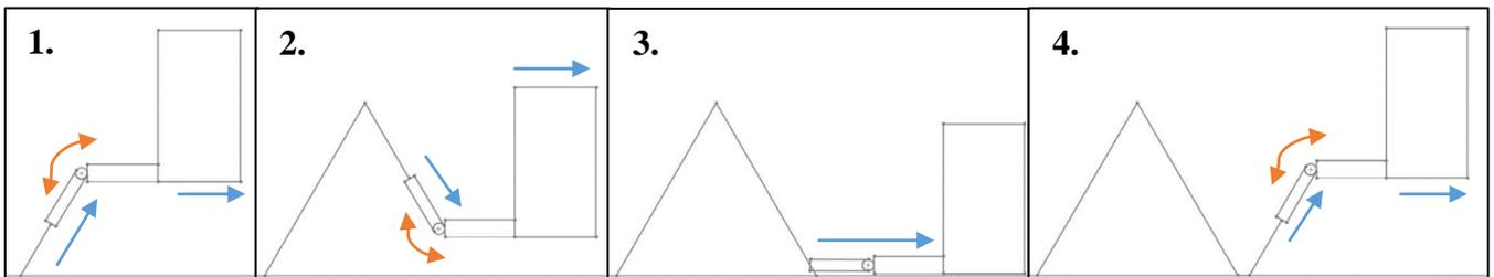
Figure 12. General motion diagram of the guided pultrusion
