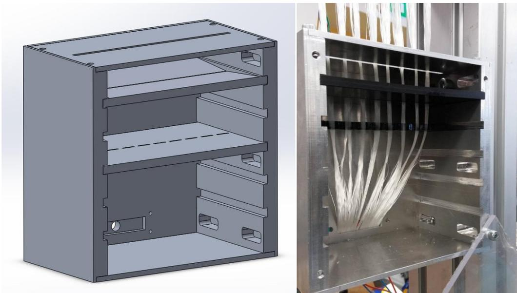
Figure 16. Resin impregnation and guiding module
