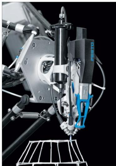
Figure 6. Festo 3D cocooner extruder [11]
