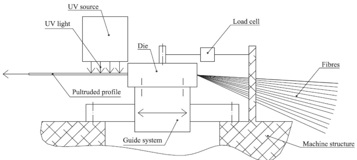
Figure 3. Pultrusion curing system with external UV light source [4]
