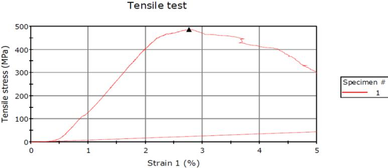
Figure 33. Tensile stress of non-cured fibers, tensile stress in MPa vs. Strain in %
