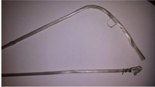
Figure 10. Manually pultruded rods
