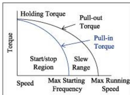
Figure 20. A general torque/speed curve of a stepper motor [34]
