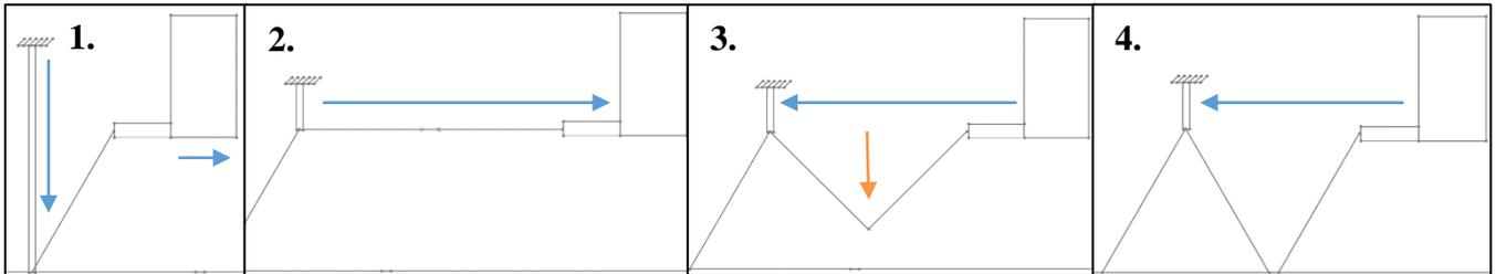
Figure 14. General motion diagram of the folding pultrusion process
