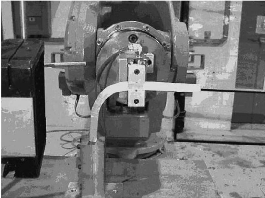
Figure 4. 6-axis robotic arm acting as the pultruder [5]
