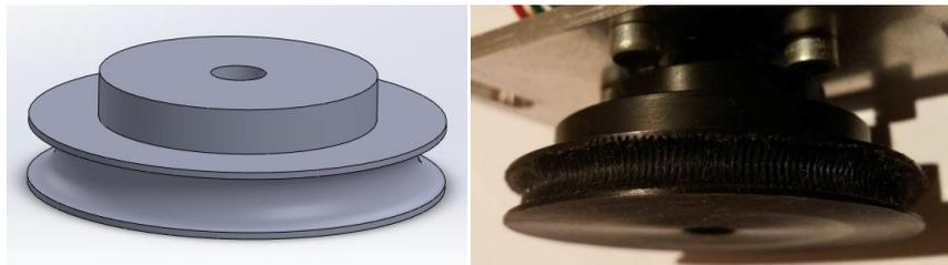
Figure 19. CAD-model of the pulling roller next to the grooved and already assembled one.
