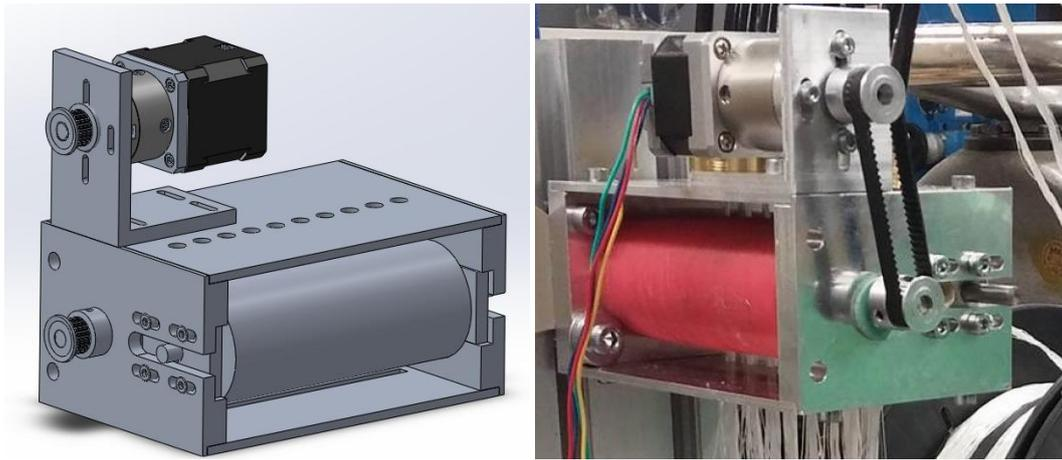
Figure 15. Fiber feeding module CAD model and implementation
