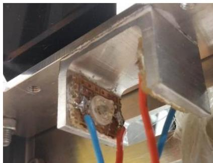
Figure 22. UV LEDs (P8D136) housed in U-profile aluminium
