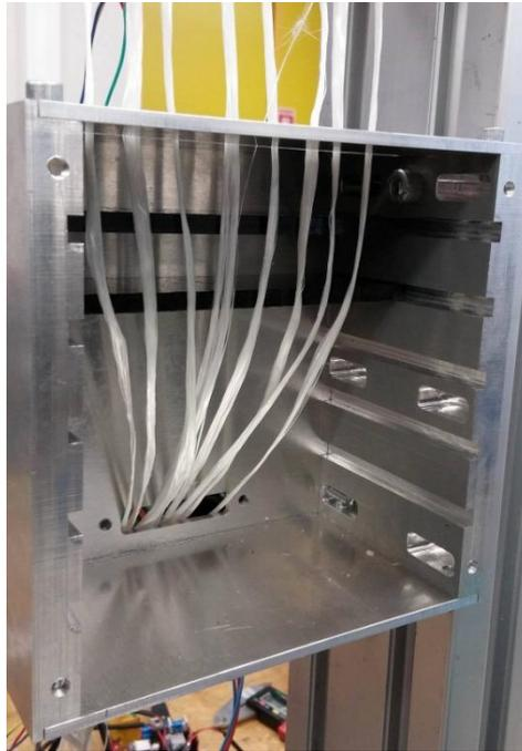
Figure 26. Guiding the fibers through the guiding and resin impregnation module.
