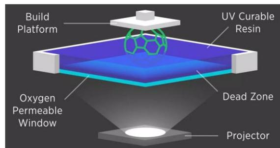
Figure 5. Continuous liquid interface production [9]
