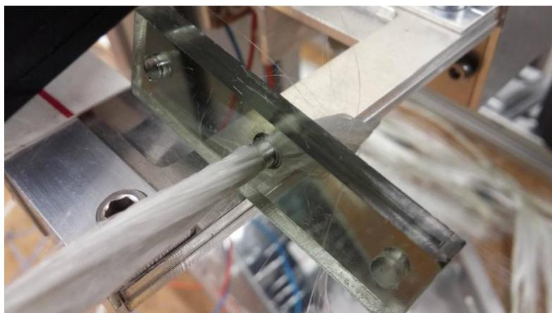
Figure 27. Fibers pulled through the die plate.
