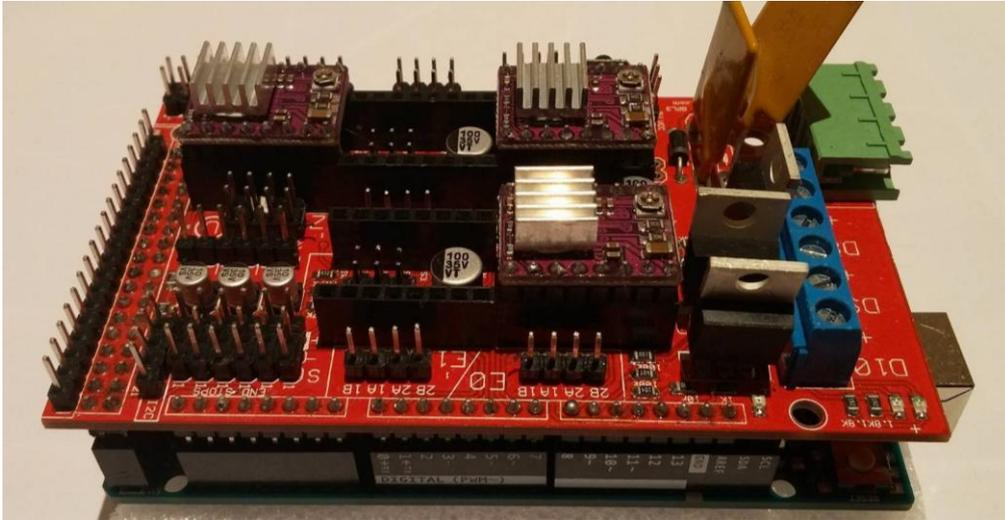
Figure 23. The assembled extension board with the Arduino Mega 2560 underneath
