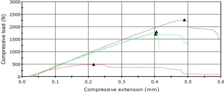
Figure 34. Compression test for 4 test specimens. Compressive load in N vs. compressive extension in mm. See also
