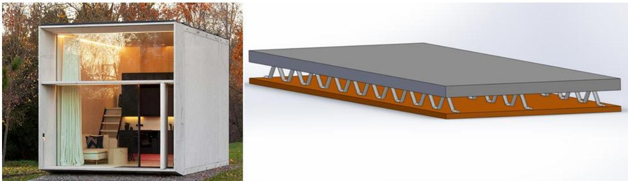
Figure 1. Modular house by Kodasema [1] and a representation of described modular wall. The main problem at hand is how to manufacture a spatial composite material structure with a constant cross-section onto a wooden panel without support elements, that could be a more efficient alternative to cutting or milling the structure from a piece of solid material, which is done at the moment, but taking into regard also the needed strength of the element.
