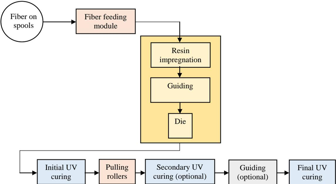
Figure 11. Block diagram of the pultrusion solution
