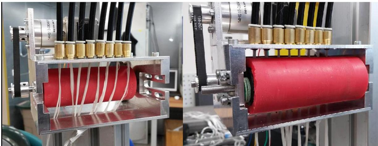
Figure 25. Guiding the fibers through the feeding module and after placing the tensioning roller.
