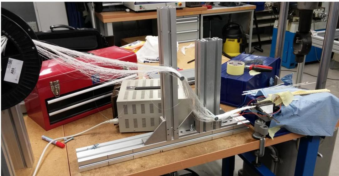
Figure 9. Pulling force test bench
