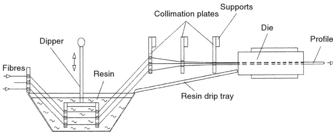
Figure 2. Resin impregnation in typical pultrusion system[2]
