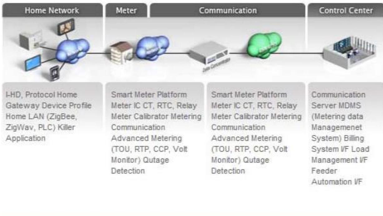
**Figure-3:** The Components of intelligent remote data collection for smart metering [15].
