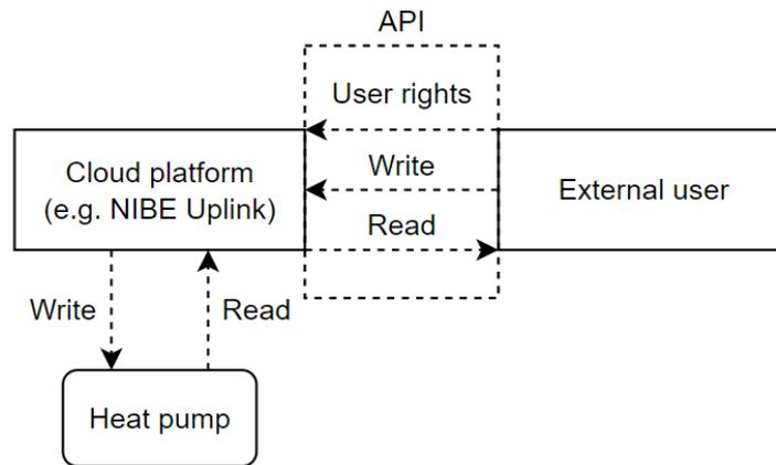
Figure 4.4 Basic principle of heat pump API
