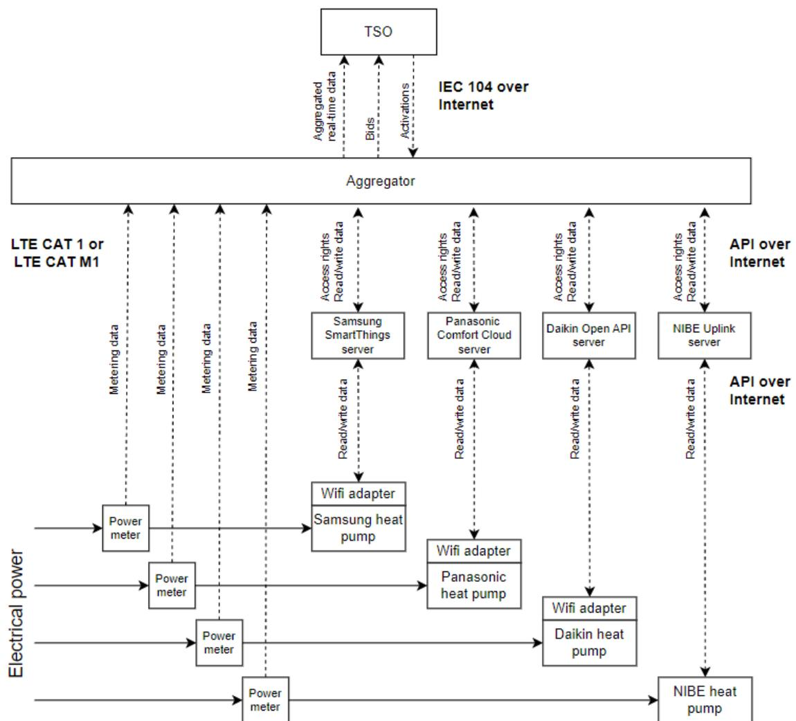
Figure 4.7 Principle diagram of the conceptual model
