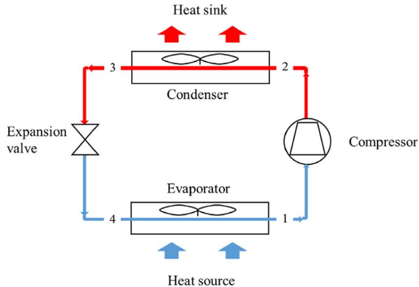
Figure 2.13 Heat pump cycle [42]
