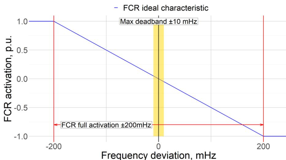
Figure 2.3 FCR activation ideal characteristic based on frequency deviation [14]
