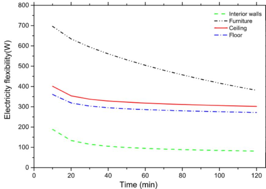
Figure 2.14 Electricity flexibility profiles of different internal mass resources [43]
