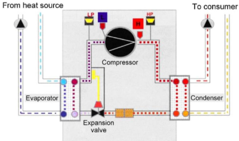
Figure 2.12 Principal diagram of heat pump [40]
