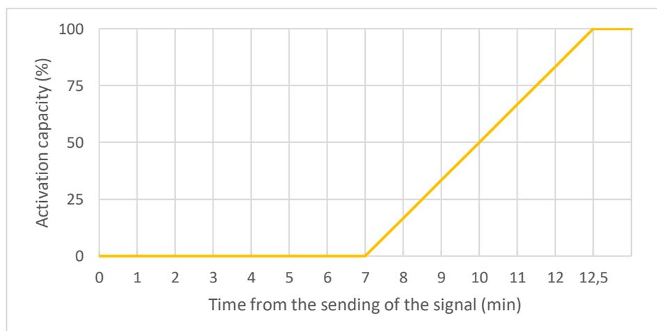
Figure 2.5 Minimum activation speed for mFRR [16]
