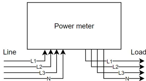
Figure 4.1 Connection diagram for direct meter
