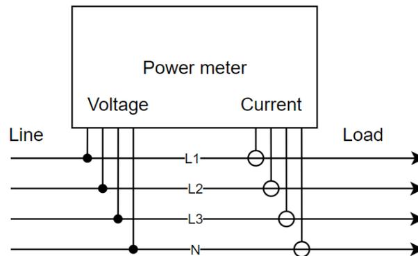
Figure 4.2 Connection diagram for power meter with current transformers
