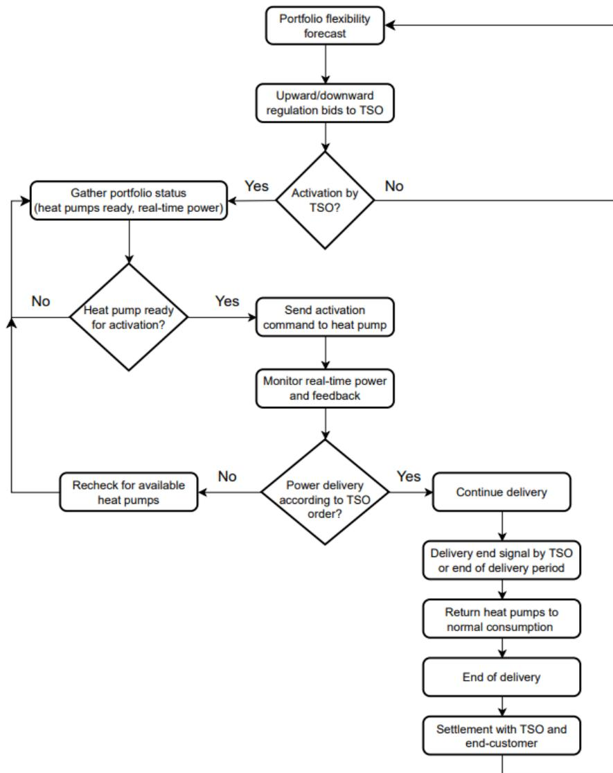
Figure 4.8 Balancing service process with heat pumps
