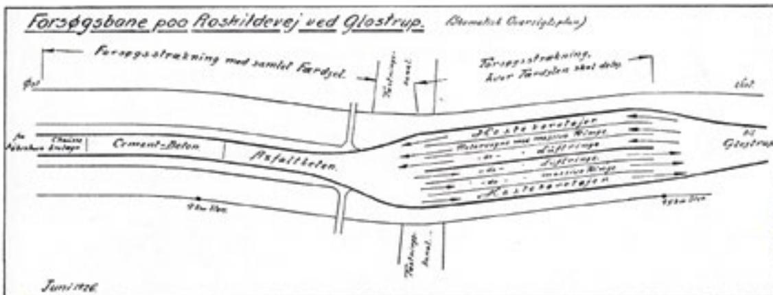
Different surfaces were experimented with on the test track along Roskildevej. The left side of the map shows marked sections of the road paved with cobblestones, cement and asphalt. (Danish Vejtidskrift)
