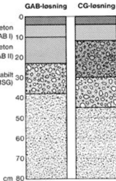
*Following remarkable scientific advancements in the 1960s, highly durable roads could be built, and heavier vehicles could be tolerated. The image shows two deep road constructions in Denmark the late 1970s; under the top asphalt layer was an additional asphalt mixture on top of a gravel layer. (from Burchardt & Schönberg)*
