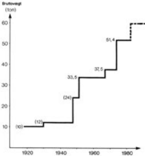
**Figure 1.** Over time, the maximum weight for vehicles has continued to rise as roads and vehicles have become better engineered. The curve shows that development in Sweden, which is representative of most other countries in Western Europe.
