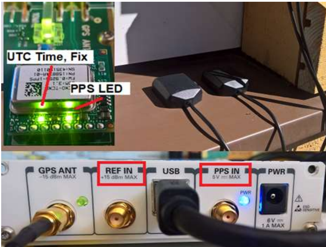
Figure 35 Synchronization capabilities on USRP B 210
