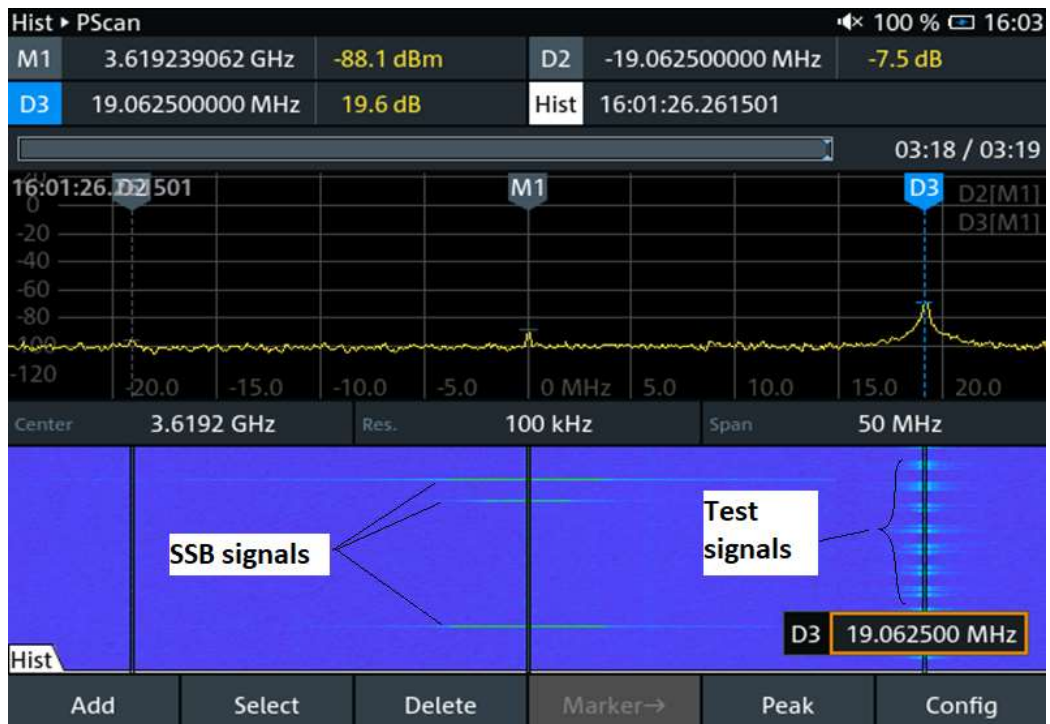
Figure 53 Test signal is generated to the upper subcarrier k = 635
