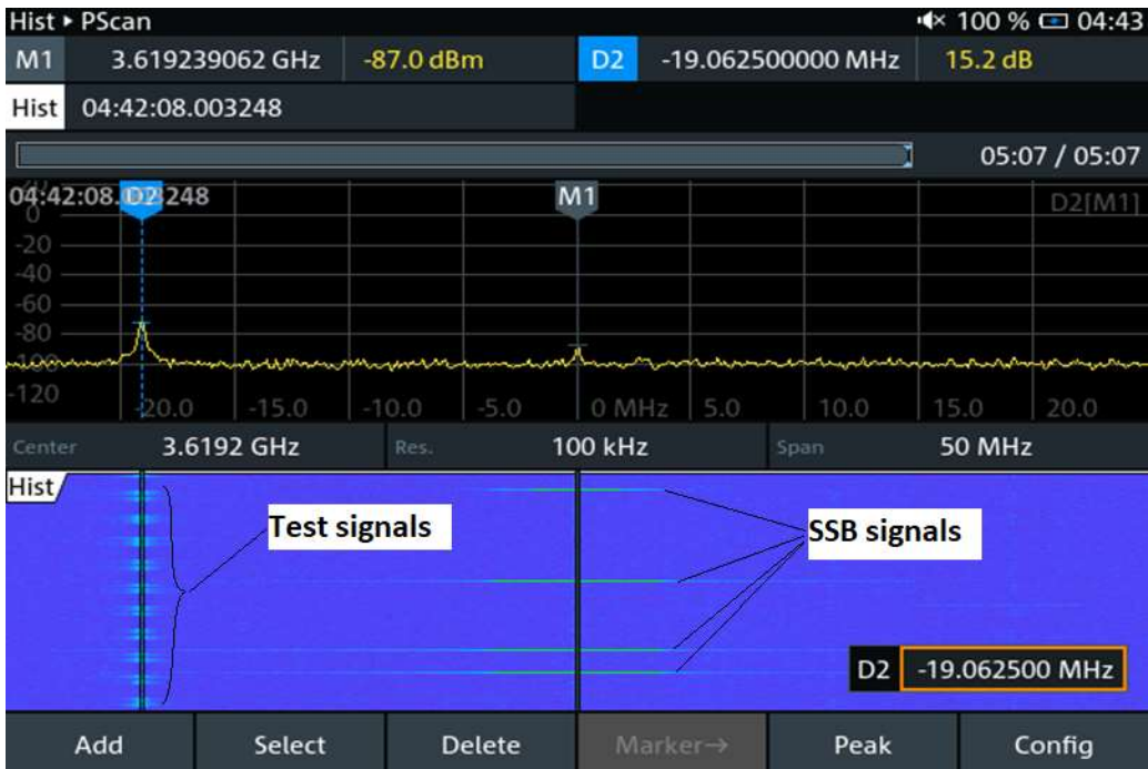
Figure 52 Test signal is generated to the first subcarrier k = 900
