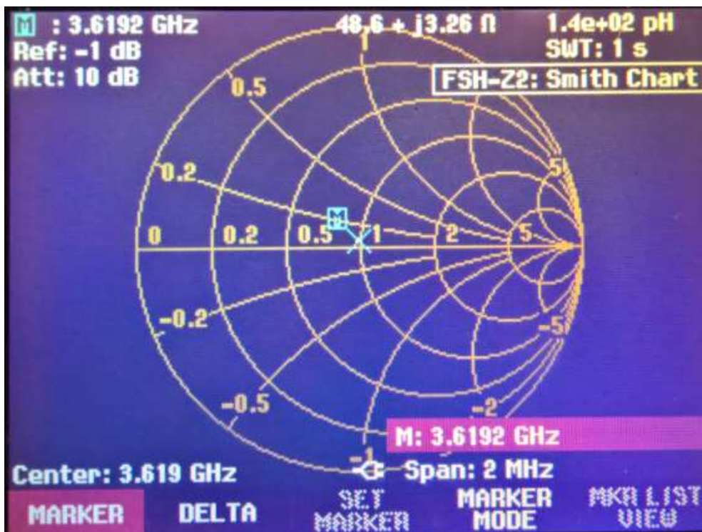
Figure 38 Antenna tuning result at f = 3619 \text{ MHz} Z = 48.6 + j 3.26\Omega
