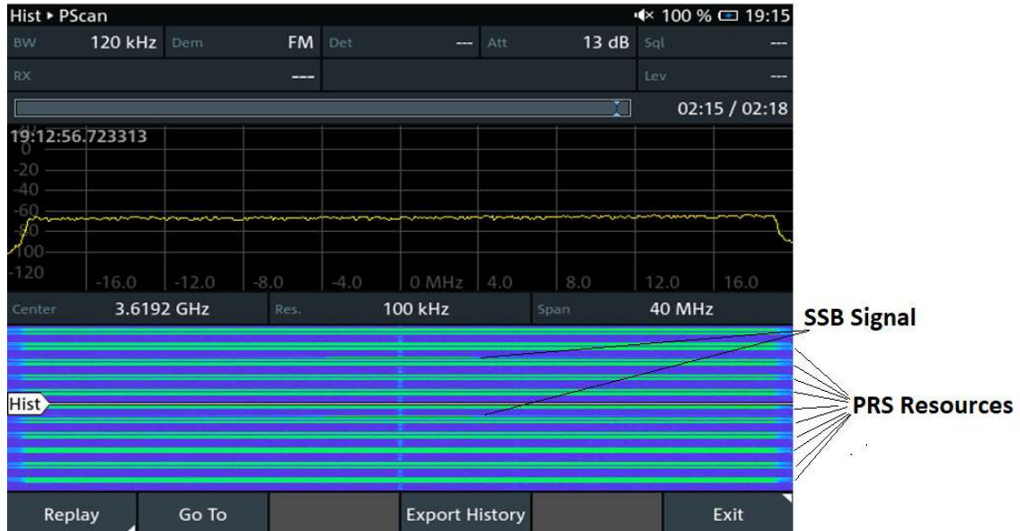
Figure 55 Captured PRS resources – all Tx slots are filled except the SSB occupied slots.
