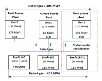
Figure 9. Expected thermal capacities to produce and utilize retort gas in Eesti Energia's energy complex after 2030.
