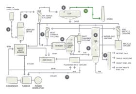
Fig.1. Process diagram of the Enefit280 oil shale retorting technology [7]
