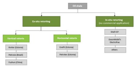
Figure 5. Oil shale retorting technologies [2].
