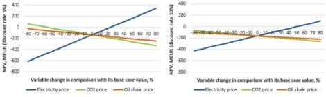
Figure 16. NPV sensitivity graphs for a potential project of an oil shale power plant.
