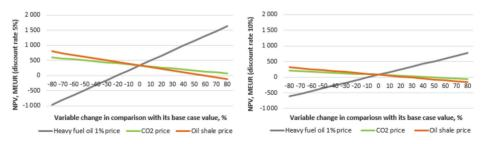
Figure 14. NPV sensitivity graphs for a potential project of a shale oil production plant.
