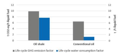
Figure 6. The life-cycle GHG emissions and water consumption of the production of liquid fuels from oil shale and conventional oil [22].
