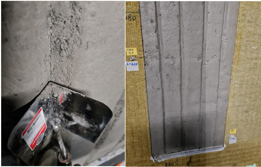
Figure 9. Four diffusion channels were grooved into PCM mortar during application for all but one experimental cross-section.
