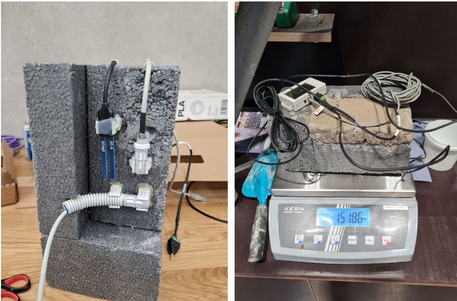
Figure 17. Small-scale sample set up for calibrating SMS for measuring PCM mortar volumetric moisture content. Besides SMS, Hobo temp sensors were used to ensure isothermal conditions of the measurements and SHT35 were used to measure RH in hygroscopic conditions.
