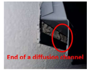
Figure 2 Cross section A-A (see Figure 1 section 2) of the test wall (left); diffusion channels pressed into fresh PCM mortar during application (right, above); air gap between steel sheets where diffusion channels reach to external environment (right, below)
