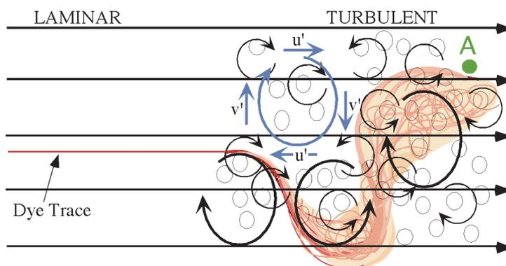
**Figure 2.** Tracer transport in laminar and turbulent flow structure. Source: Massachusetts Institute of Technology (Open Courseware).
