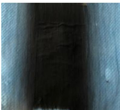
Figure 2.2 Example of electrospun nanofiber mat containing polymer, ionic liquid and carbon additives
