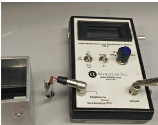
Figure 2.4 Conductance measuring device
