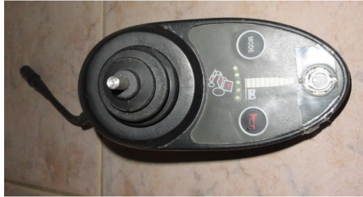
Figure 5.16. The Joystick that controls the main track, the three work-mode push-buttons
