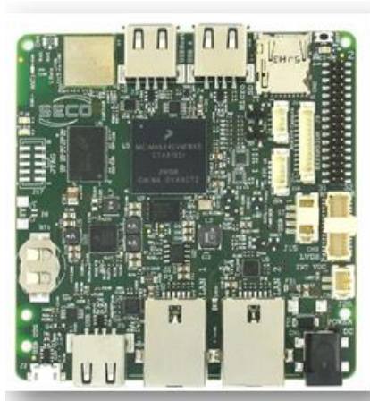
Figure 5.1. Freescale i.MX6 single-board pc
