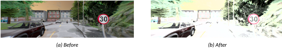
Figure 66: Camera view of attack case 1: before (a) and after (b) the implementation of the Strong Light Exposure Attack.
