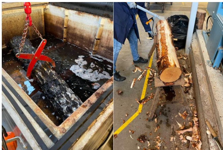
Figure 3.1 Soaking and debarking of peeler logs
