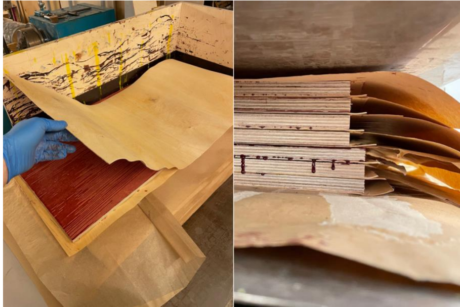
Figure 3.7 Layup and cold-pressing of face veneers on core plywood panels
