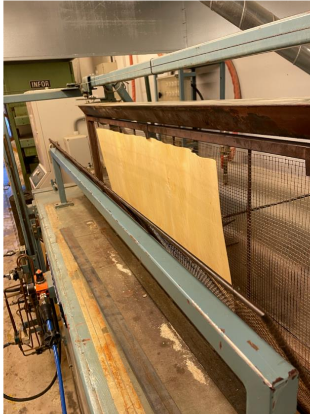
Figure 3.4 Veneer drying with air circulation veneer dryer
