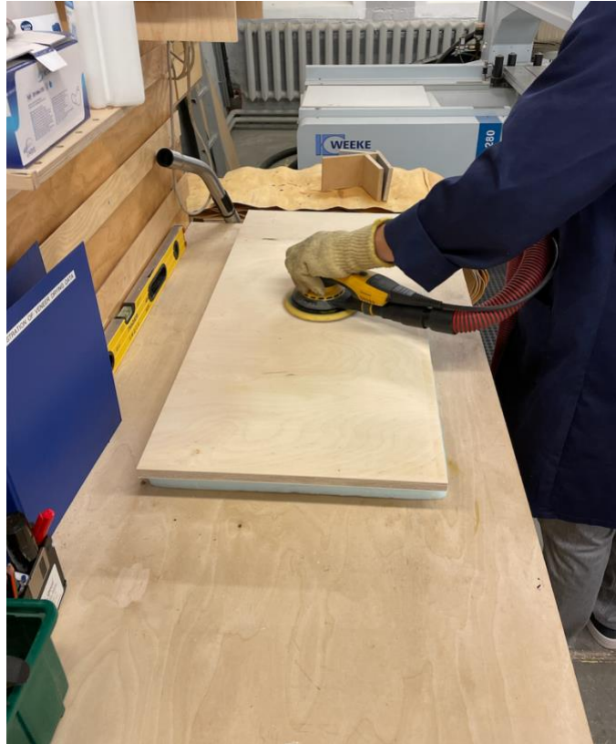
Figure 3.8 Panel sanding with rotary sanding machine
