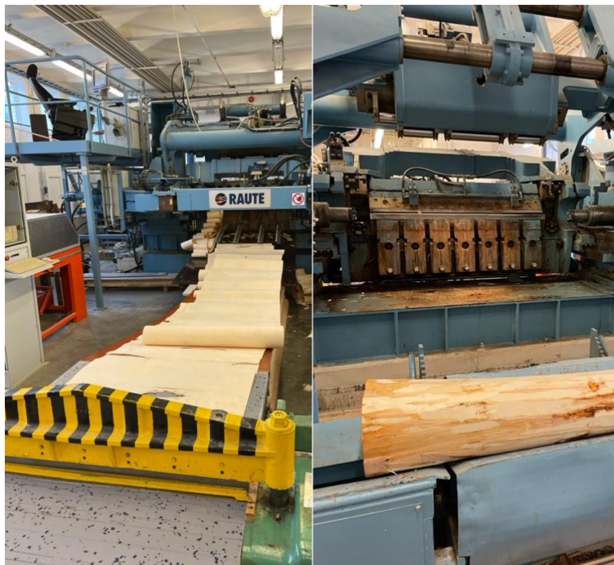
Figure 3.2 Peeling of logs with Raute peeling lathe
