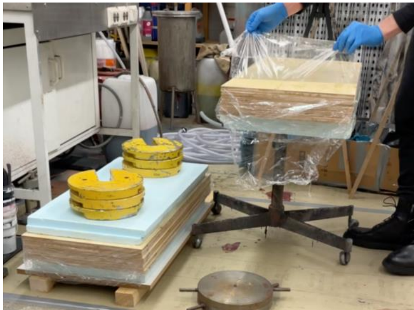
Figure 3.10 Stacking of the FR-treated plywood panels with polyethylene film separation
