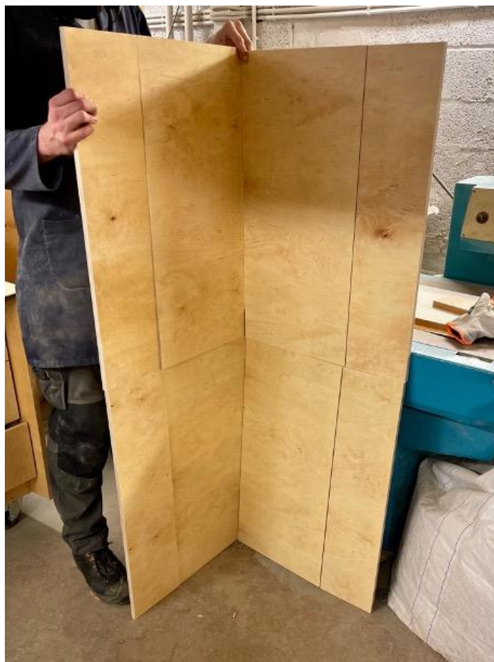
Figure 3.15 Illustration of assembled specimen for the SBI test
