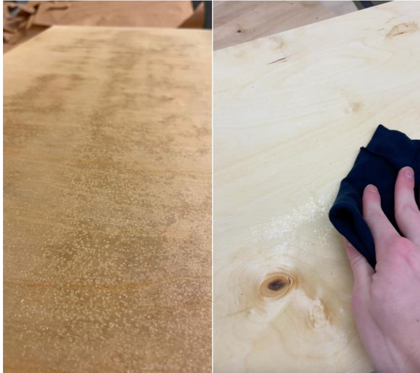
Figure 3.11 Residual fire retardant salt crystals and their removal from panel surface
