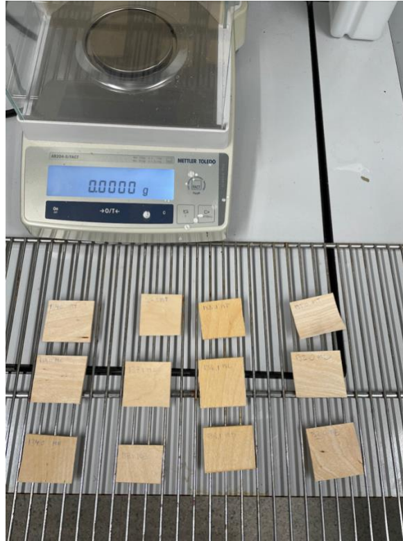
Figure 3.5 Determination of veneer moisture content
