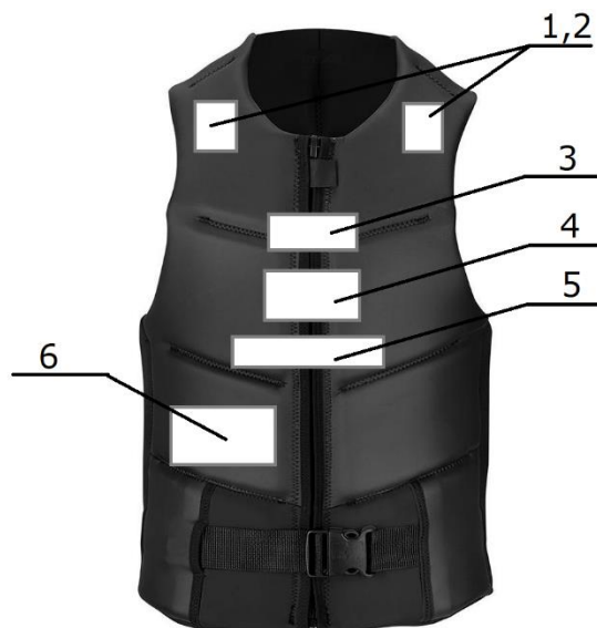
Figure 6 – main components proposing location (1,2 – audio and vibration modules, 3 – camera, 4 – Raspberry Pi, 5 – ultrasonic modules, 6 – accumulator)
