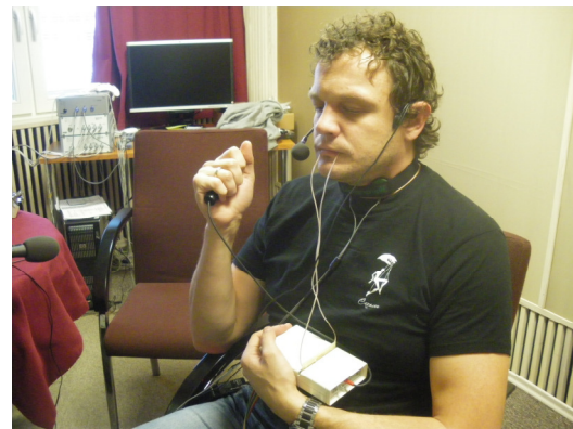
Figure 2. The subject wearing electrodes of the EGG system, the EPG palate, and a close-talking microphone
