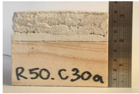
Figure 6-11. Test specimens prepared for the cone heater tests in TP3: Left – 10 mm thick lime plaster with a reed mat on timber specimen; Right – 30 mm thick lime plaster without reed mat.
