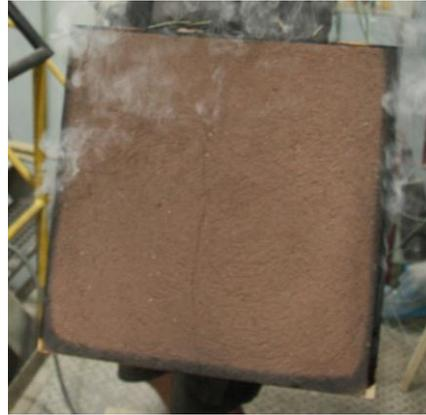
b) Test 9b – Plaster system ClaySF04.
