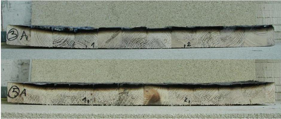
Figure 6-43. The cross-section of timber panels protected by 30 mm thick plasters:
