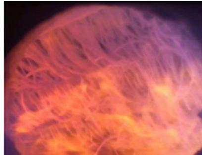
b) Test 4 – Reed board exposed to fire after the fall-off of plaster system.
