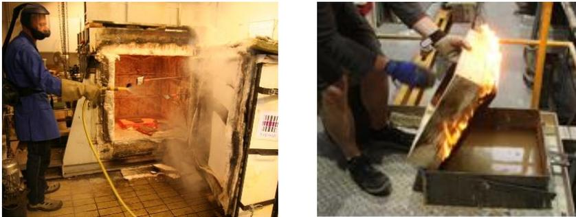
*Figure 5-21. Cooling down the test specimens after its removal from furnace:
