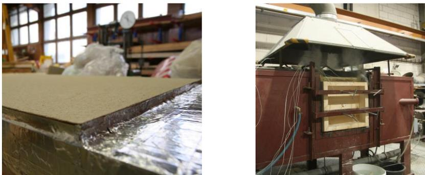
*Figure 5-20. Preparation of test specimens for furnace testing: Left – Sides of plaster fixed with aluminum tape; Right – Test specimen fixed in furnace in TP3.*
