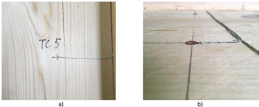
Figure 5-16. Close-up on the fixation of thermocouples (TC) on the exposed side of the timber elements before the application of plaster systems: a) TP1 and TP2; b) TP3 and TP4.
