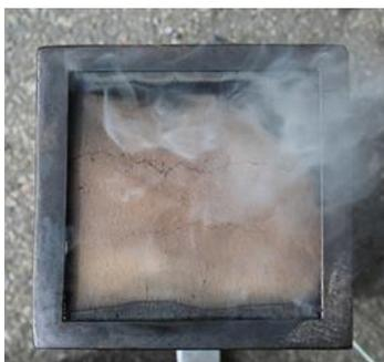
c) View of the plasters' surface after its removal from furnace and before extinguishment
