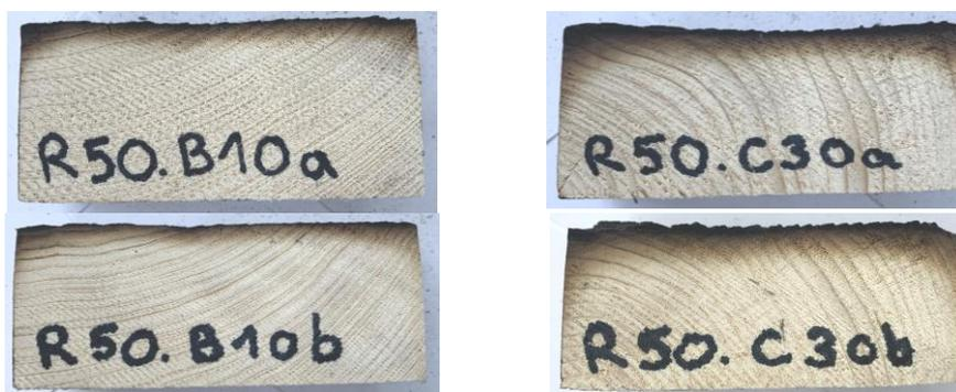
Figure 6-16. Residual cross-sections of timber specimens (50 mm) from double-testing after cone heater tests when protected by plaster: Left – 10 mm lime plaster; Right – 30 mm lime plaster.
