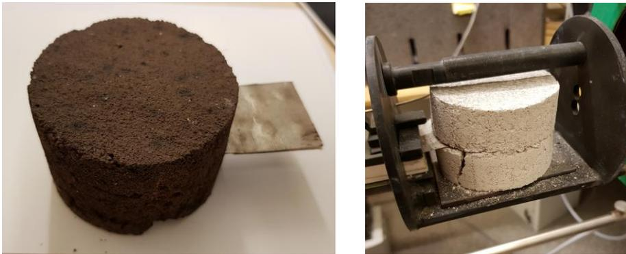
Figure 5-6. Documentation of test specimens after TPS tests: Left – Close-up of ClaySU04 after testing; Right – Cracking of LimeSU04 when tested in the electric furnace.
