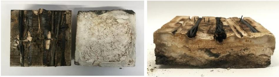
Figure 6-13. A test specimen after cone heater testing and cooled down with water: Left – Top view of the timber specimen from which the plaster system was removed and put aside; Right – A close up of the plaster system (incl. the reed mat), placed upside down.
