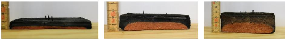
Figure 6-3. Cross-section of clay plasters placed upside down, after cone heater testing.
