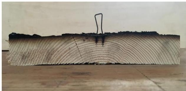
b) Close-up of a timber plank of a timber panel with a pulled-out staple.
