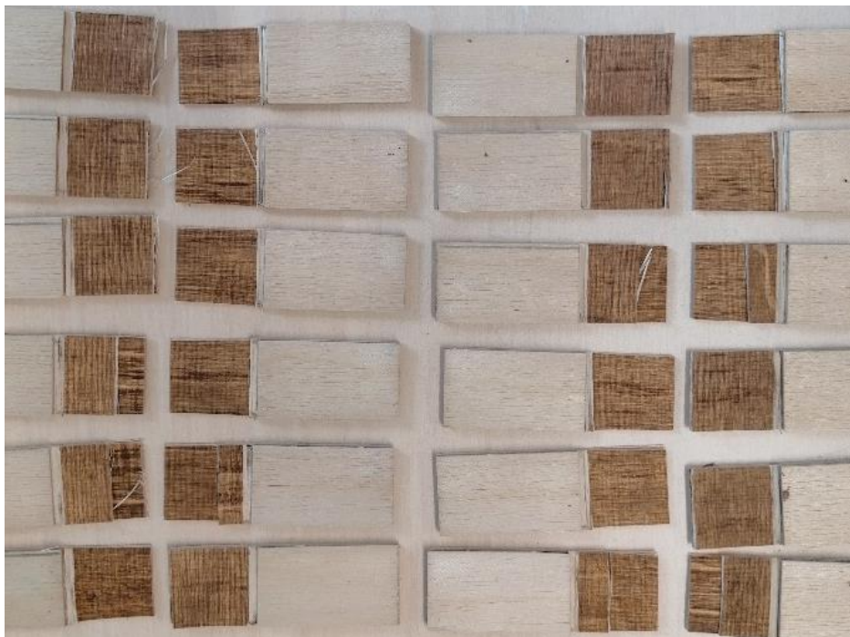
Figure 3.11 Shear strength specimens after testing, panel nr 11 (bond shear strength: 0.9 MPa; adhesive: LPF; wood species: aspen; log soaking temperature: no pre-soaking)
