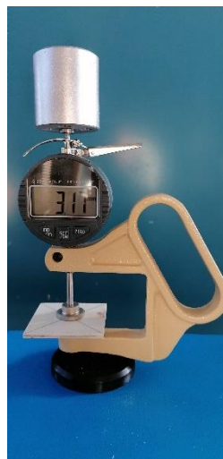
Figure 2.4 Plywood thickness measuring on density specimen
