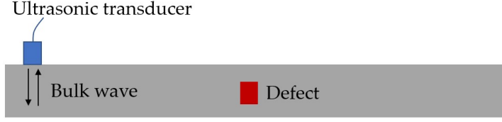
Figure 5: Schematic diagram of ultrasonic bulk wave testing.
