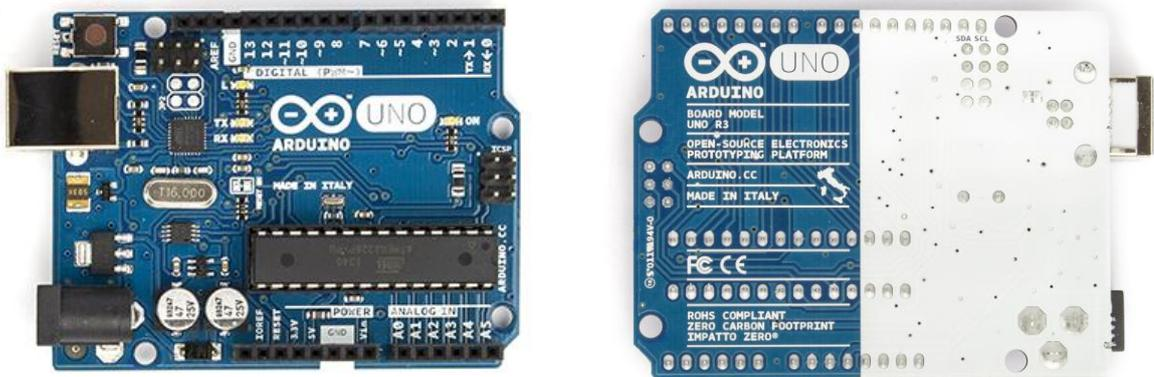
Figure 26. Top and bottom side of arduino Uno (image taken from arduino.cc).
