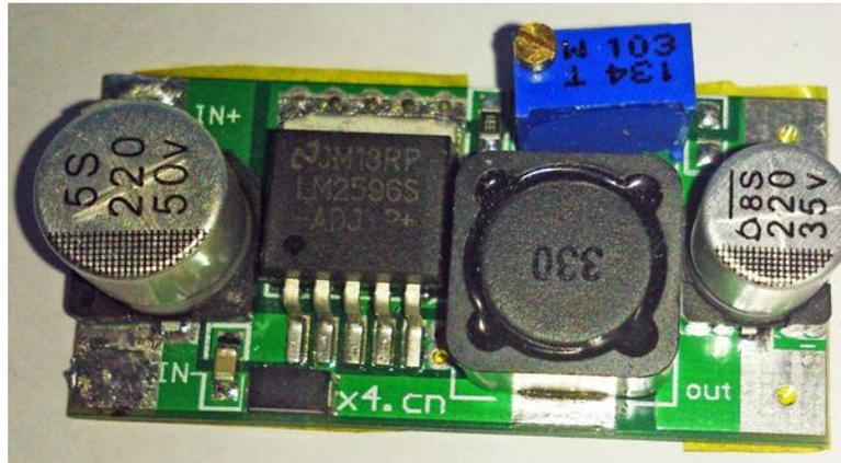
**Figure 31.** Step down voltage convertor
