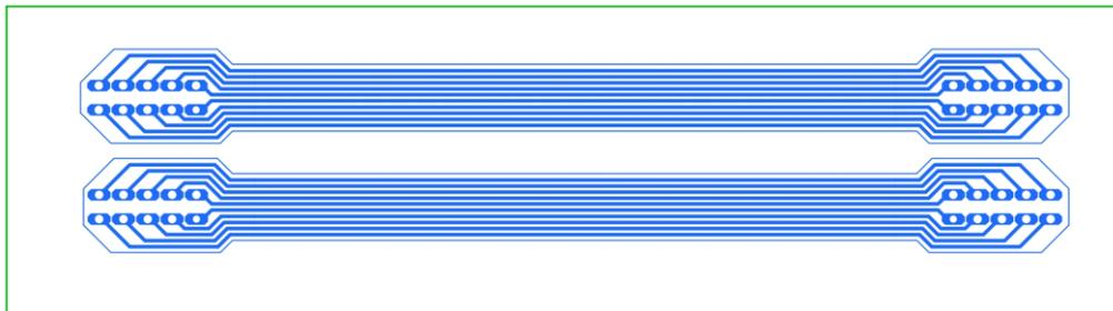
**Figure 34.** Flexible flat cable
